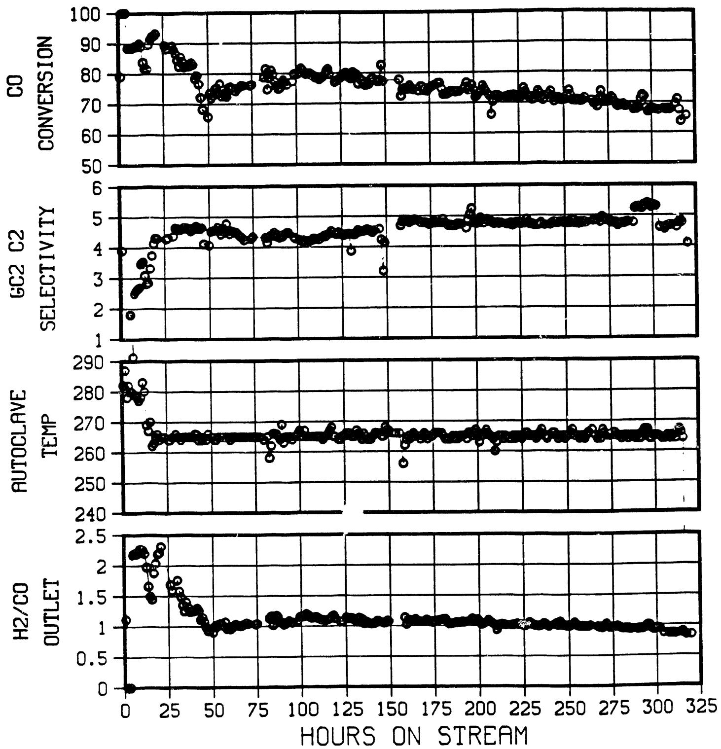
PRECIPITATED IRON CATALYST 6616-37 IN SLURRY AUTOCLAVE
