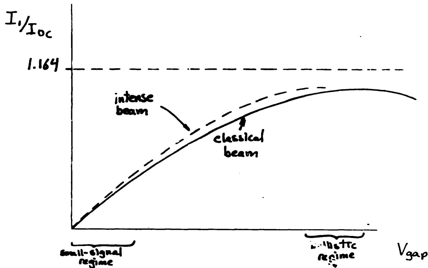
Current modulation always less than 1.164 if beam has space charge
