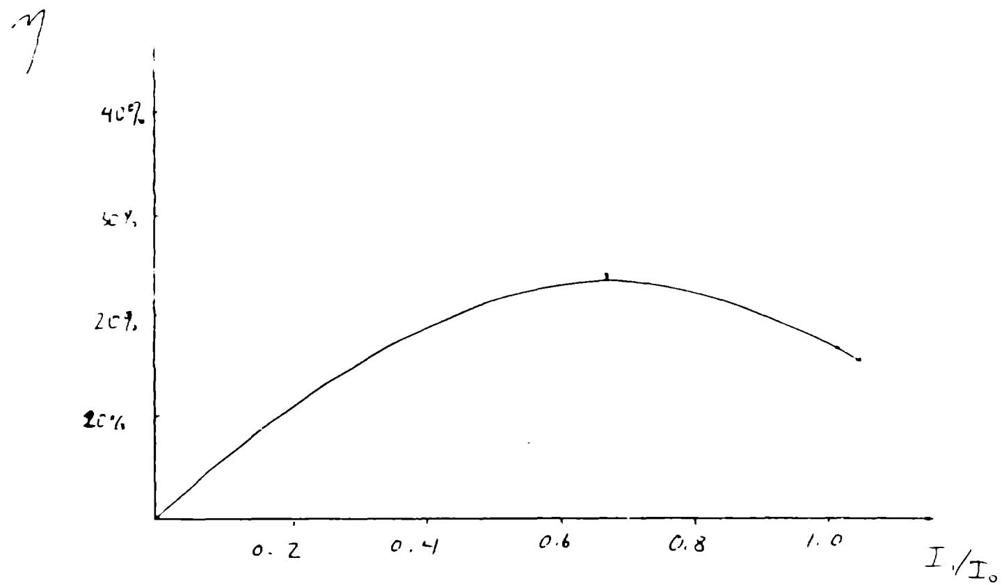
Fig. 11 Extraction efficiency for a 500kV, 52A RKA versus harmonic bunching with  $r_{in}/r_{in} = 114$
