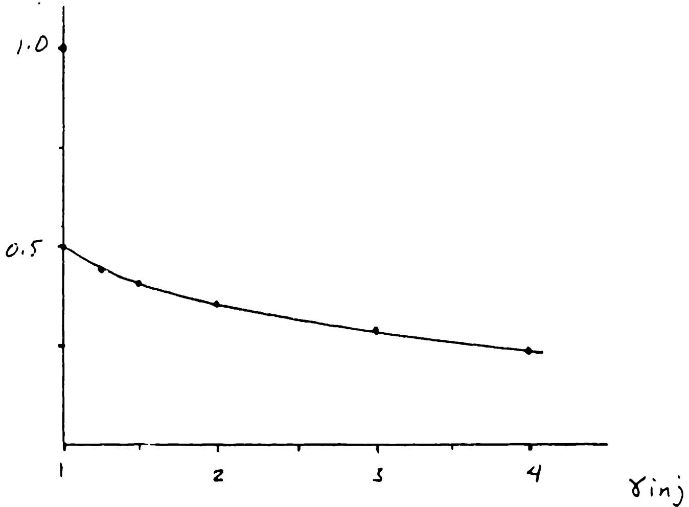
Fig 11 Ratio of Kinetic Energy to Potential Energy for Maximum current transmission for different Injection Energies
