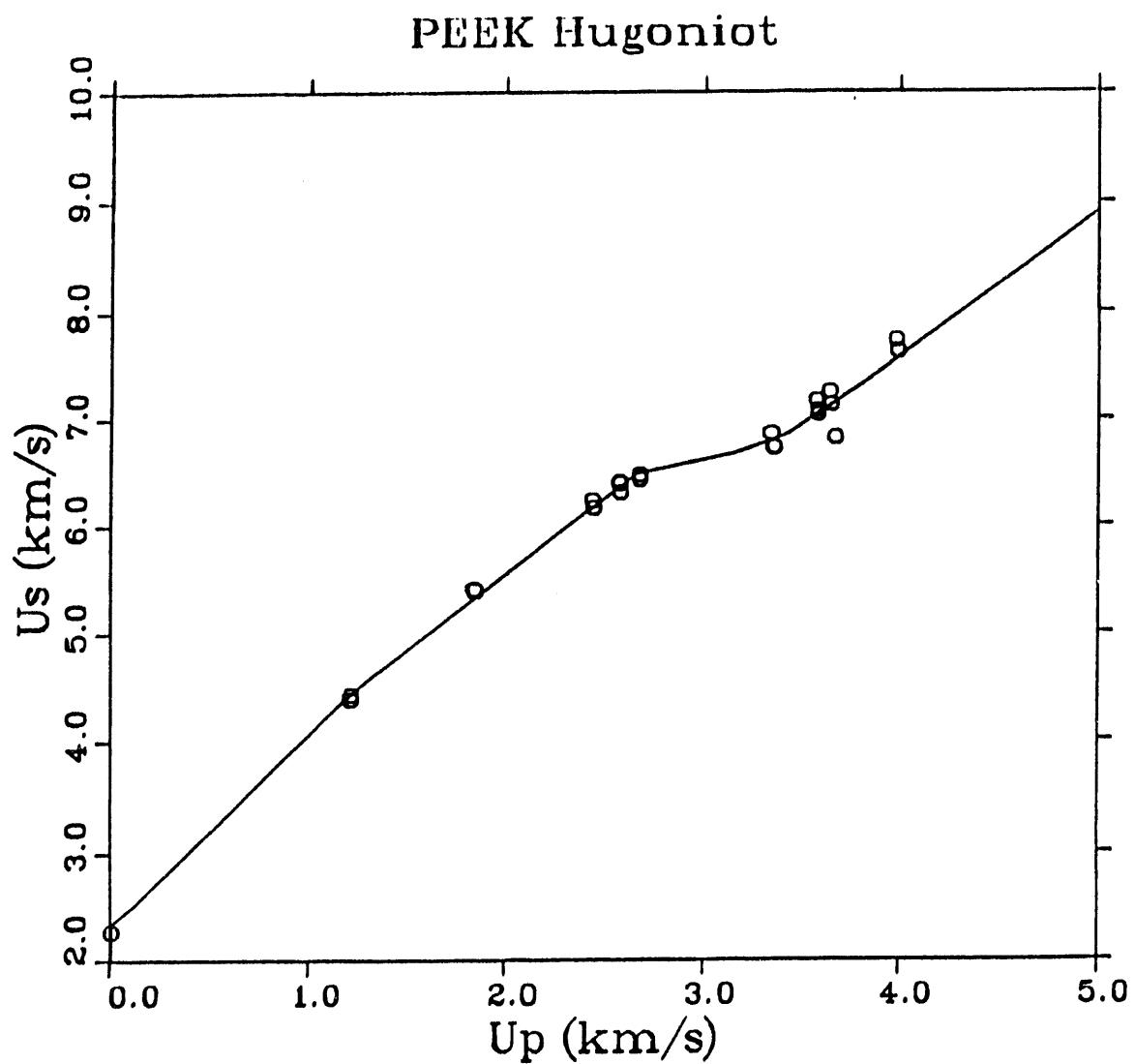
Figure 1. The theoretical Hugoniot for PEEK is compared with Hugoniot data from Ref. 14.
