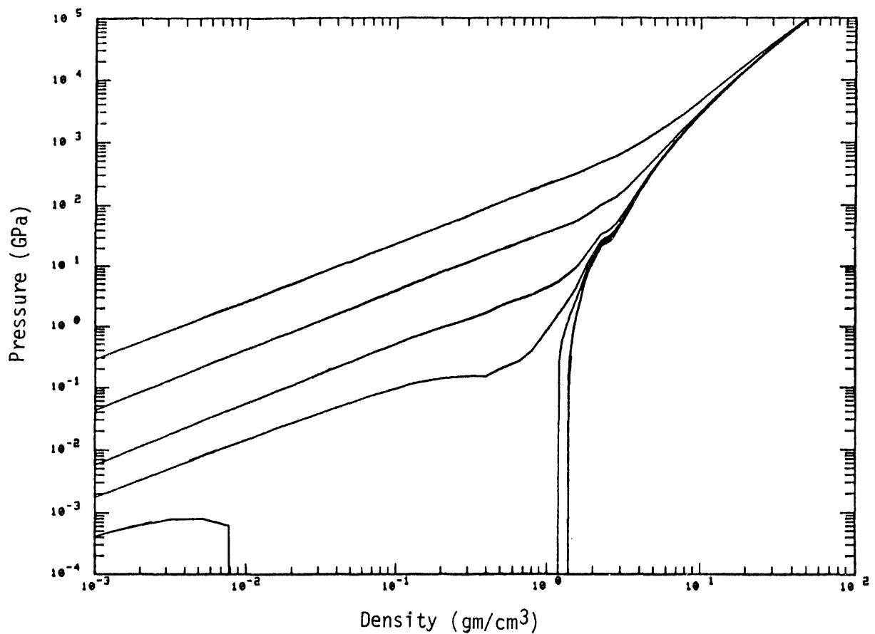
Figure 2. Selected isotherms from the theoretical SESAME EOS for PEEK. The temperatures included are 0 K, 1000 K, 2050 K, 5000 K, 25000 K, and 100000 K.
