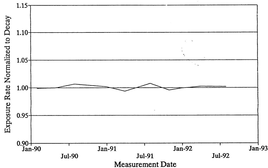
Figure 2 - Constancy Verification Results for Shepherd  $^{137}\text{Cs}$  Gamma Irradiator
