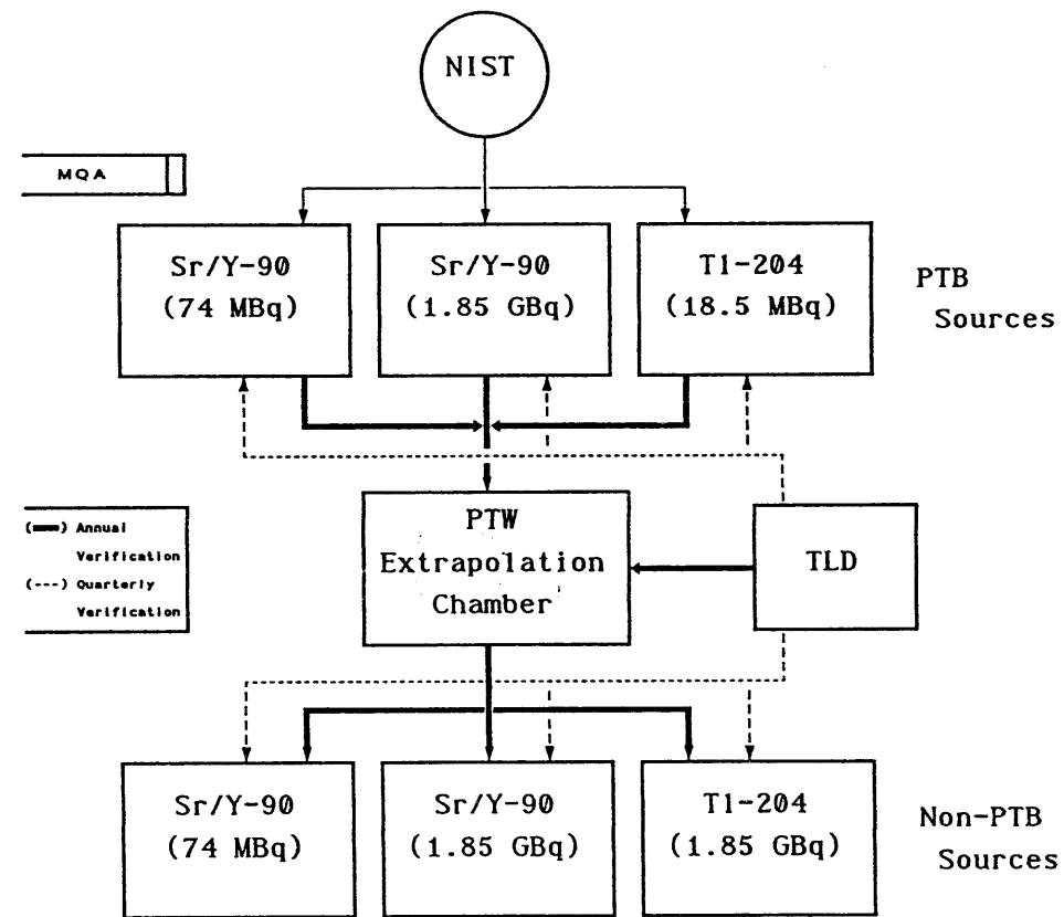
*Figure 5 - Pathway for Maintaining and Verifying the Traceability of Beta Radiation Fields*
