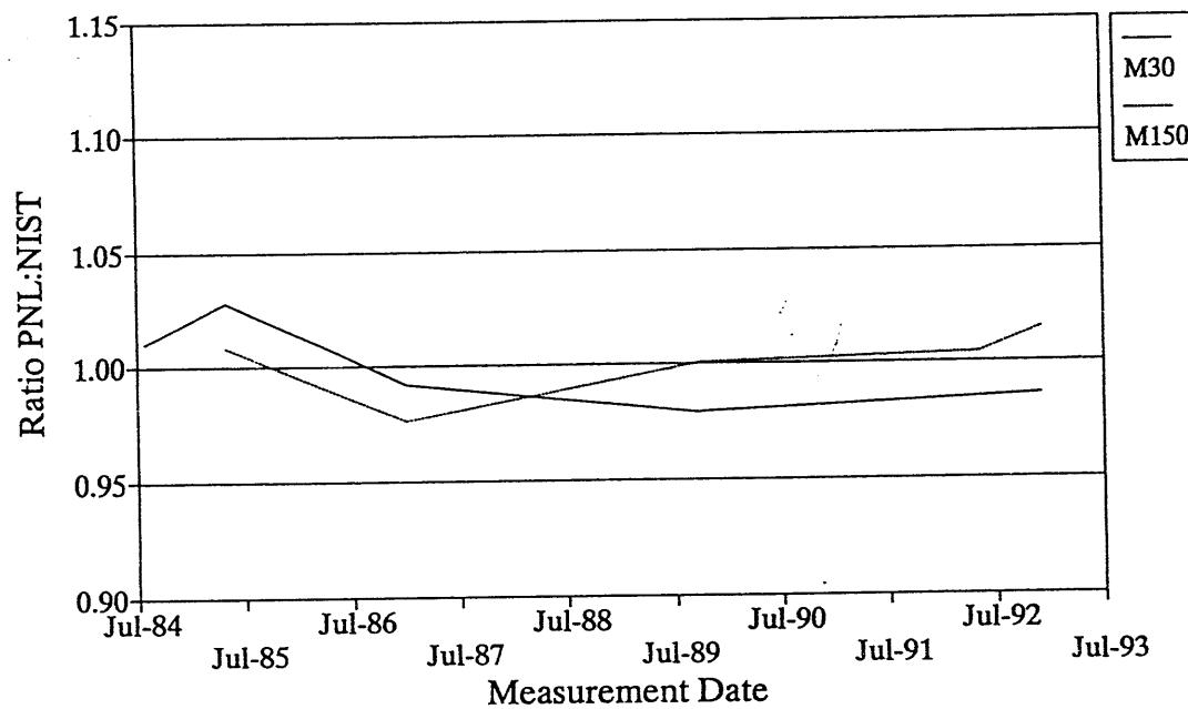
Figure 4 - Comparison of PNL and NIST MQA Results for M30 and M150 Bremsstrahlung X-Ray Techniques
