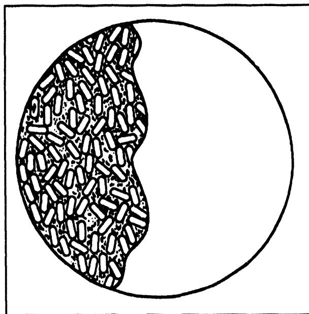
Figure 2.4a. Biobeads are formed by mixing heat-killed bacteria with a polymer.
