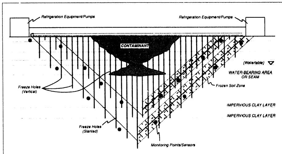
Figure 1.6. Frozen Soil Barrier at a Non-Arid site; cross-sectional view.
