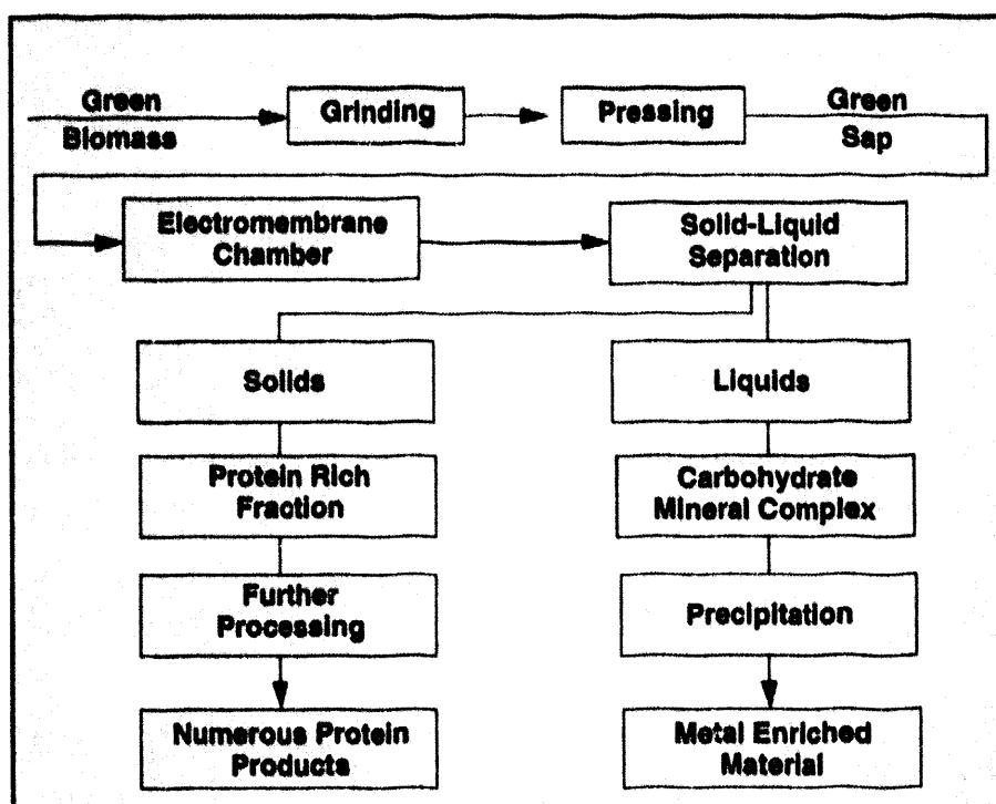
Figure 2.5. Fractionation Separation Technology Process for Macrophyte Remediation of Contaminated Soils.
