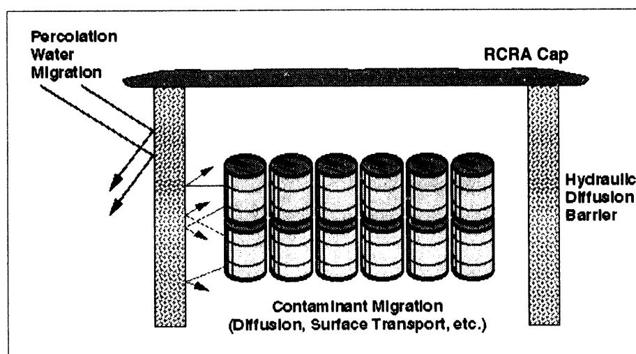
Figure 1.5. Reduction of contaminant migration and mobility using hydraulic/diffusion barriers.
