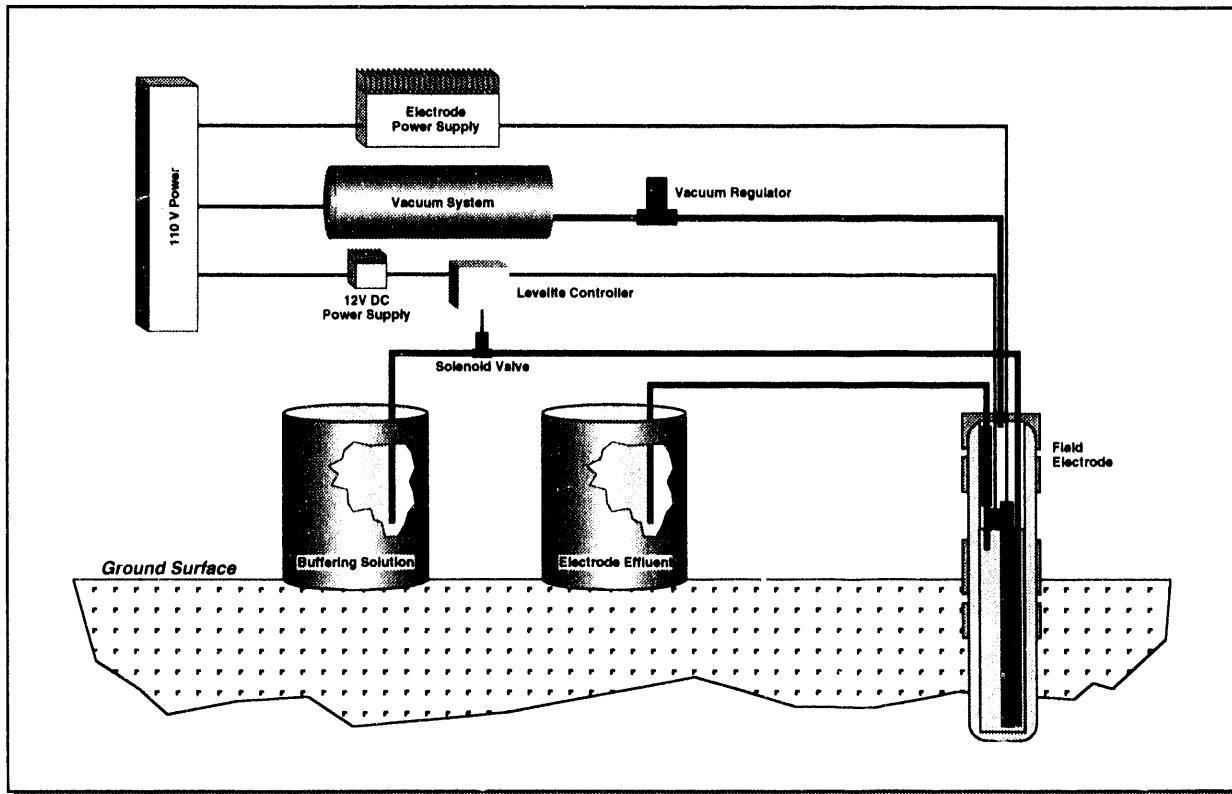
Figure 4.0. Electrokinetic Migration Technology (Sandia).
