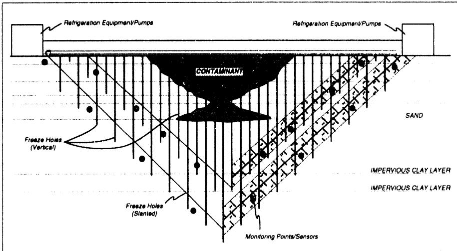
Figure 1.7. Cryogenic Barrier at an Arid site; cross-sectional view.
