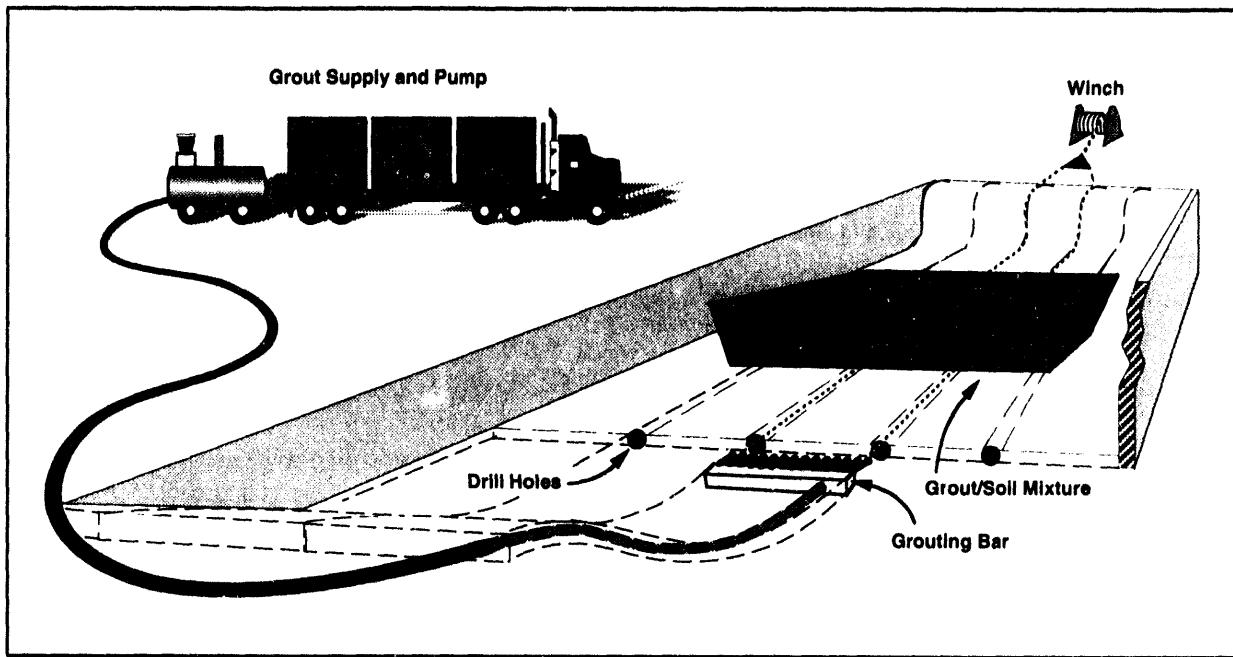
Figure 1.8. Containment vault formed in place using grouting bar.
