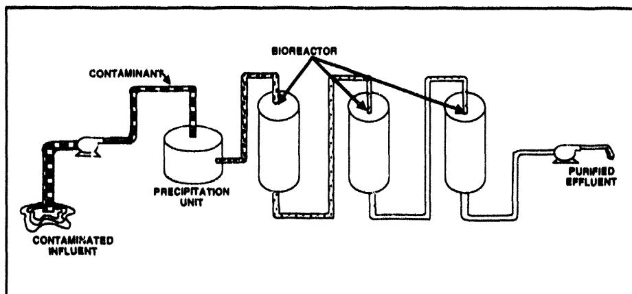
Figure 2.4b. Contaminated water is passed through a series of bioreactors.
