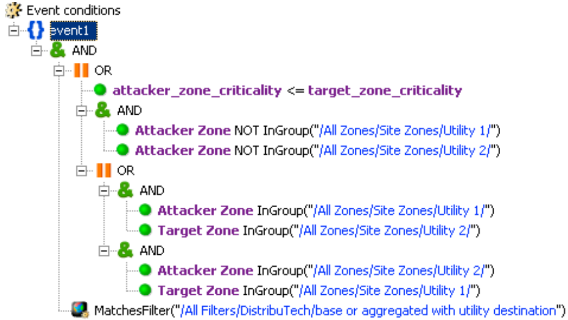
Figure 12. ArcSight filter for potential network traversal events
