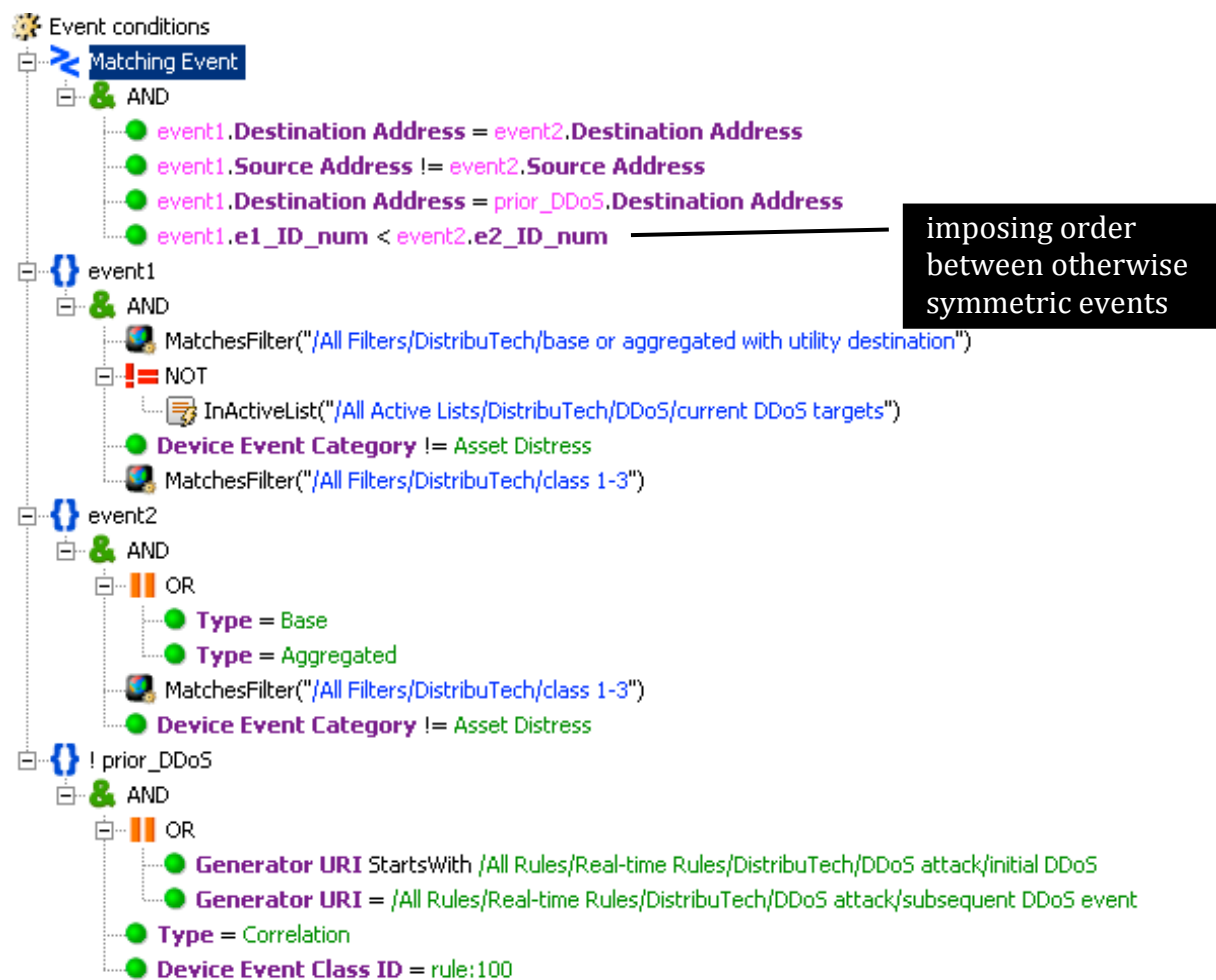
Figure 11. ArcSight Rule definition for DDoS Case 3
