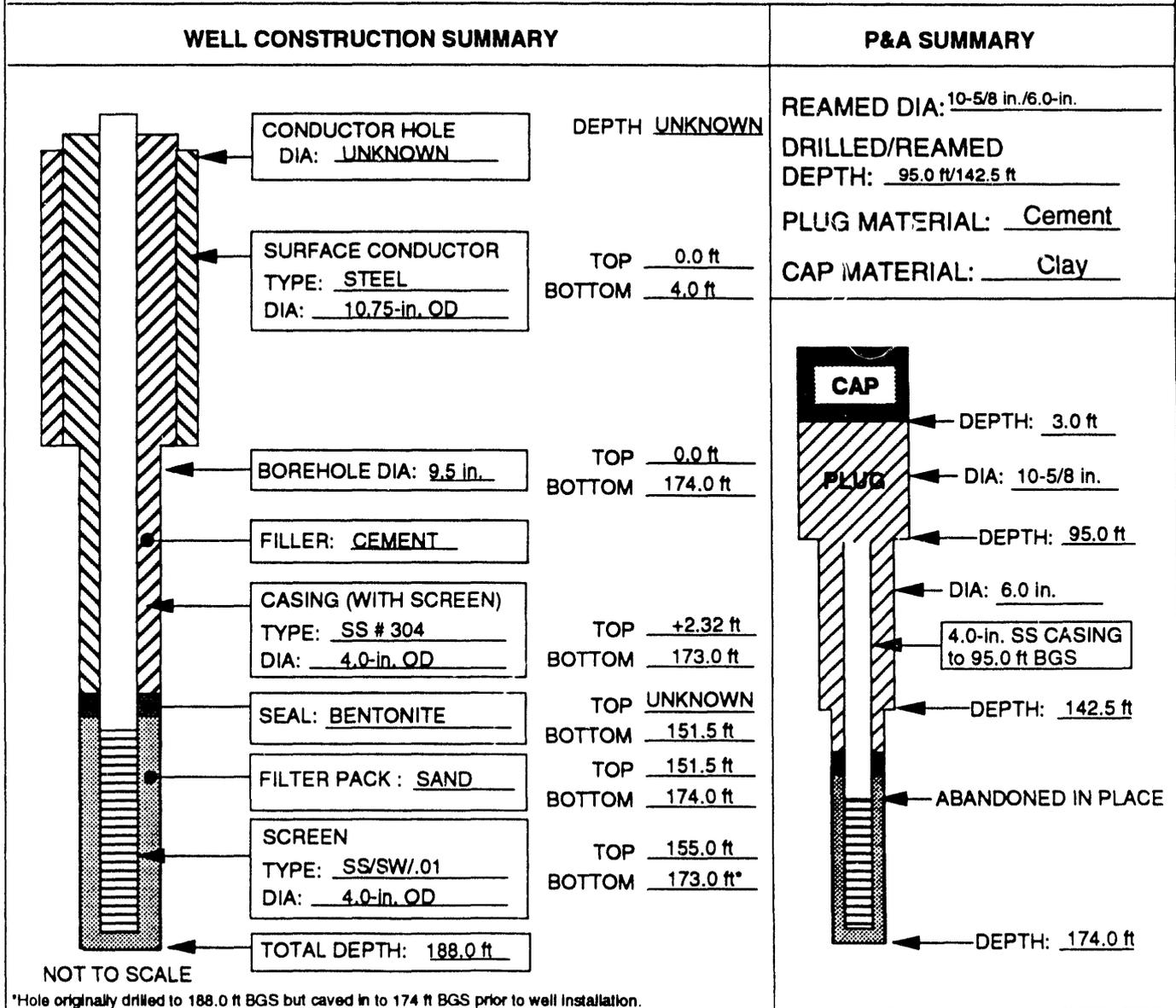
\*Hole originally drilled to 188.0 ft BGS but caved in to 174 ft BGS prior to well installation.
