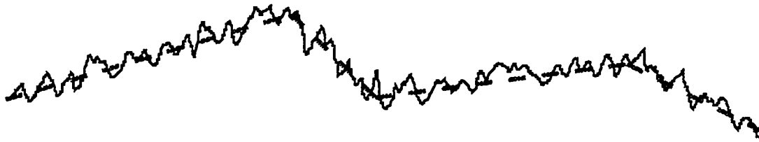
Figure 3: Sketch of a rough faceted surface. In addition to the high-frequency roughness, much larger facets, represented by the dashed lines, are also visible. The DWBA may fail for such surfaces.
