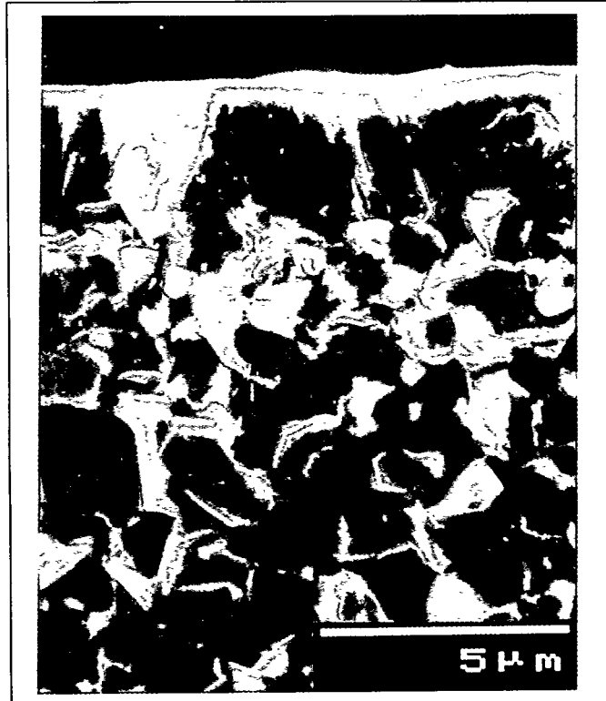
Figure 8: Fracture surface of LC102 heated to 1350°C
