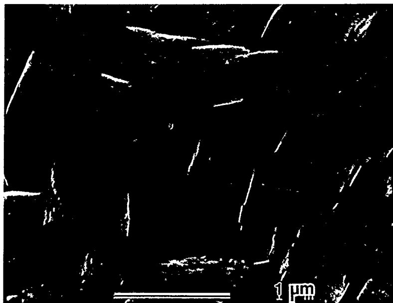
Figure 1.---SEM micrograph of the surface of as-deposited EZA coatings containing a bulk iron content of 8 w/o shows 500 nm wide crystallites and 30-50 nm wide ledges.
