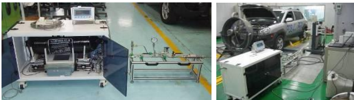
Figure 19: Weight measurement equipment for fuel economy test.
