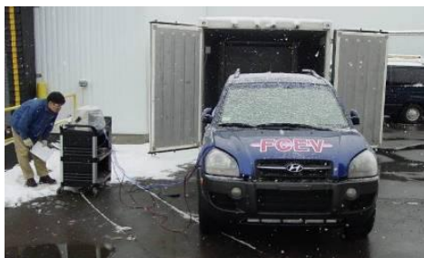
Figure 22: Cold performance test at UTCV in Connecticut.
