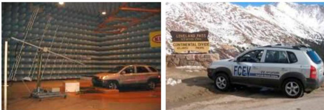
Figure 24: EMS test at HMC and high-altitude test in Colorado.
