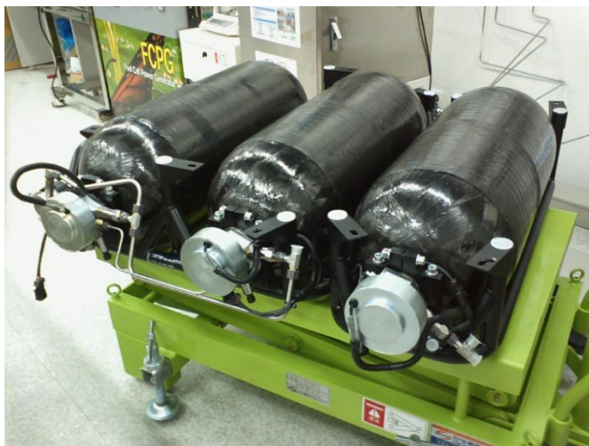
Figure 11: Gen II 700 bar hydrogen tank system.
