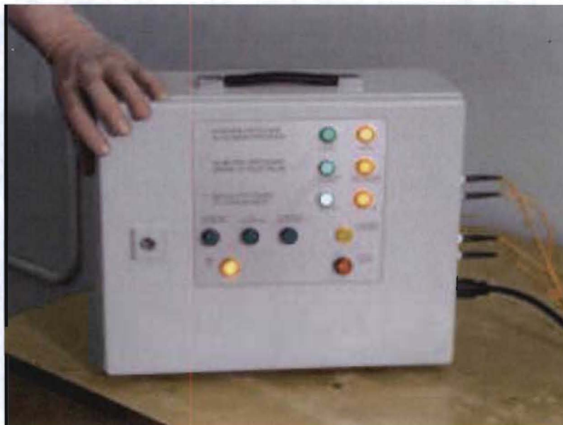
Fig. 11. The operator's control panel and display. The three pairs of red and green lamps on the upper right indicate whether or not an item being measured meets each of the three attributes.
