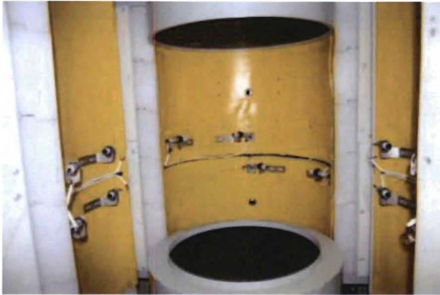
Fig. 7. Optical sensors located within the cavity of the neutron detector to detect the presence of a modified AT-400R container.
