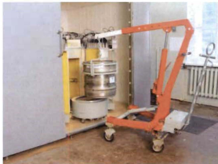
Fig. 8. Hydraulic AT-400R loading system. AT-400R containers (both modified and unmodified) are placed on the lower graphite reflector of the NMC. This reflector is mounted on wheels, which allow it to be moved into the remainder of
