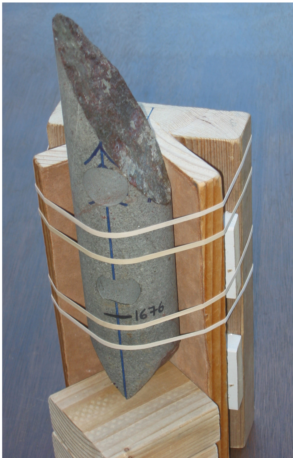
Figure 2.3. Photograph of 6.2 cm diameter oriented core segment from well 62-21 held in fixture for fracture and striation measurements. Note the two core plug holes from the paleomagnetic orientation process, the sample depth (in feet) and the blue MOL line. The upper core plug was drilled into the MOL and the lower core plug, exhibiting a rough irregular edge, was drilled from the opposite side.
