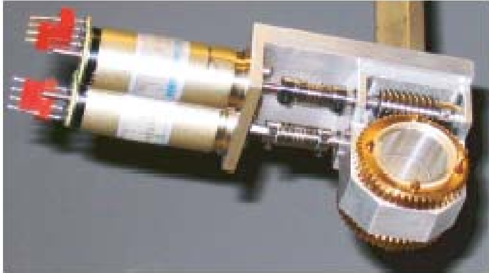
FIG. 3: Picture of the "Double wedge setup" for spatially encoding of the neutron beam.
