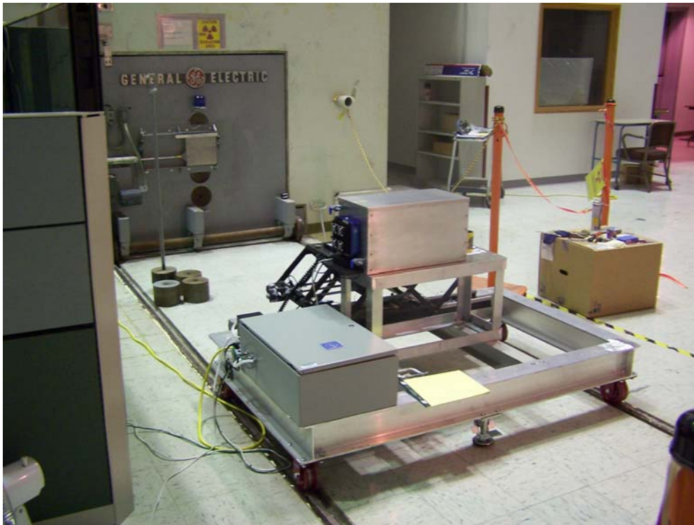
Figure 3. Rail cart assembly and thermal column door (southeast view).
