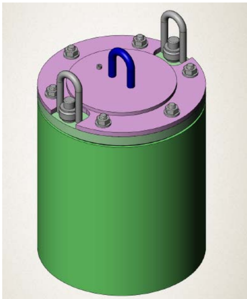
Figure A.2. Sketch of a Proposed Shielded Cask Concept
