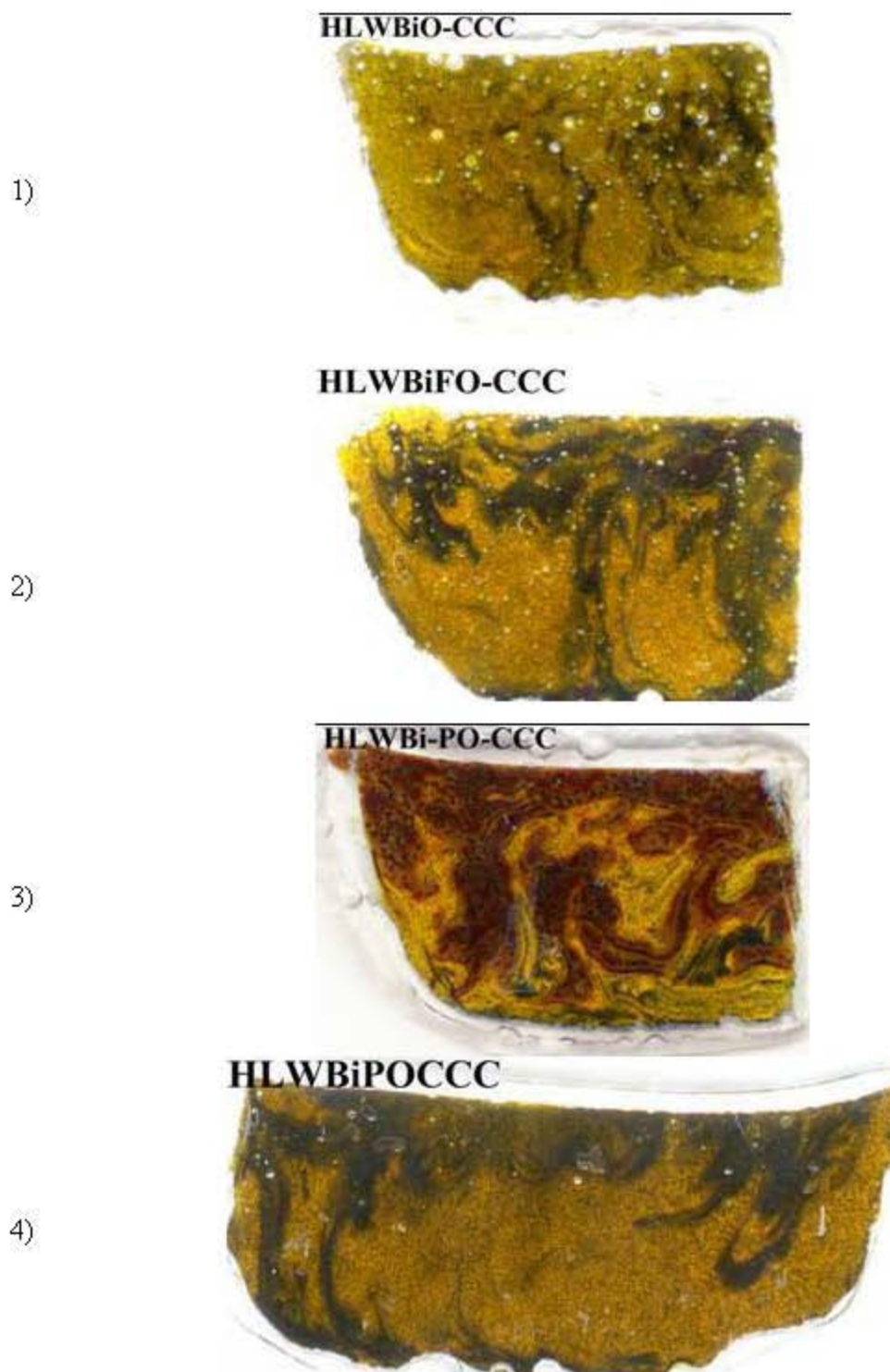
Figure 3.3e. 1) Scanned image of thin section of HLW-Bi-BiO after CCC; 2) Scanned image of the thin section of HLW-Bi-F0 after CCC; 3) Scanned image of the thin section of HLW-Bi-P0 after CCC; 4) Scanned images of the thin section of HLW-Bi-BiP0 after CCC.
