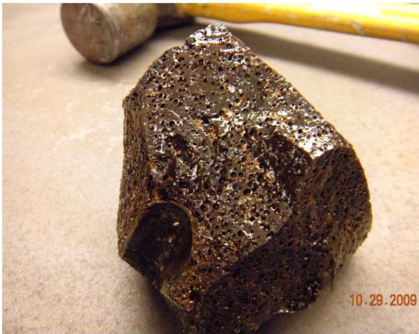
Figure 5.11.b. Foam in discharge glass G-12P-53A.
