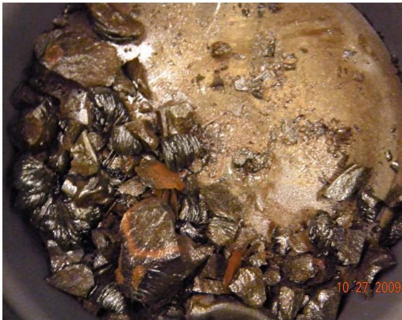
Figure 5.9. Discharge glass G12O-150A. Foam observed.
