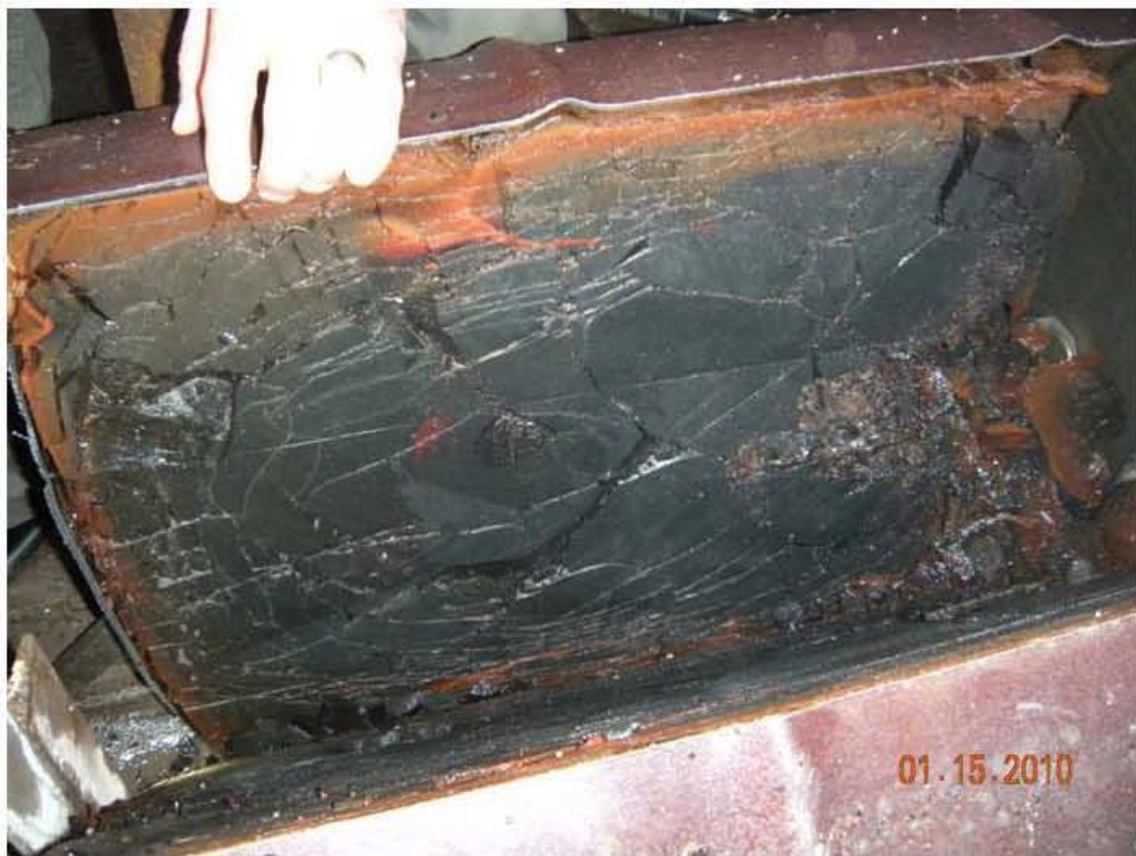
View into left half of drum, partial split.
