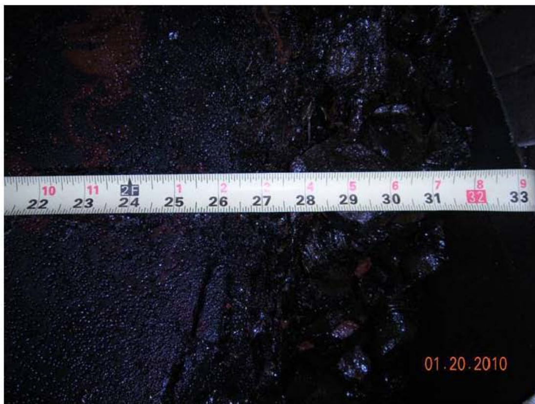
Glass measured @ center line of right half of drum.
