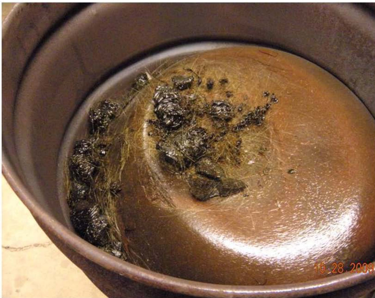
Figure 5.10. Discharge glass G-12P-32A. Foam observed.
