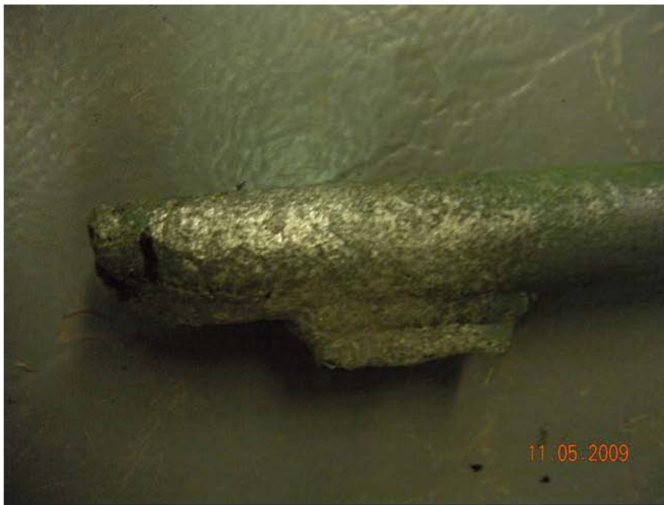
Figure 5.35. Bubbler (DB-4) tip after exposure to the high bismuth glass.
