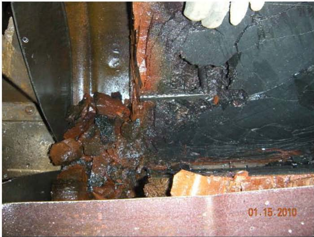
View into right half of drum showing void area, partial split.
