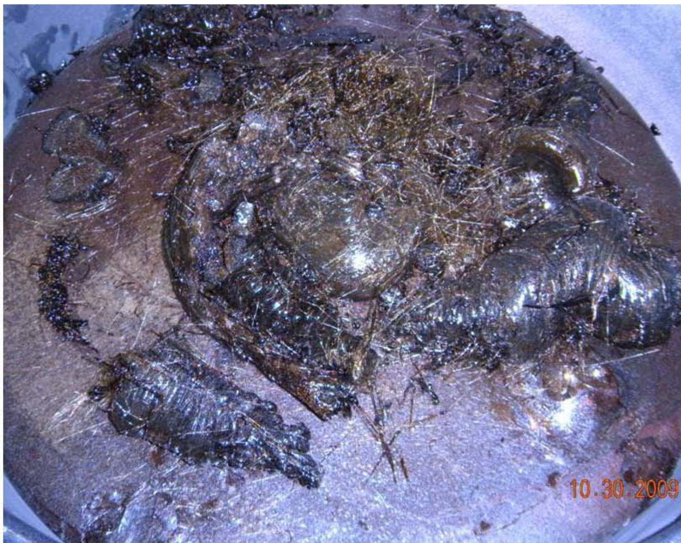
Figure 5.13. Discharge glass G-12P-88A. Foam observed.
