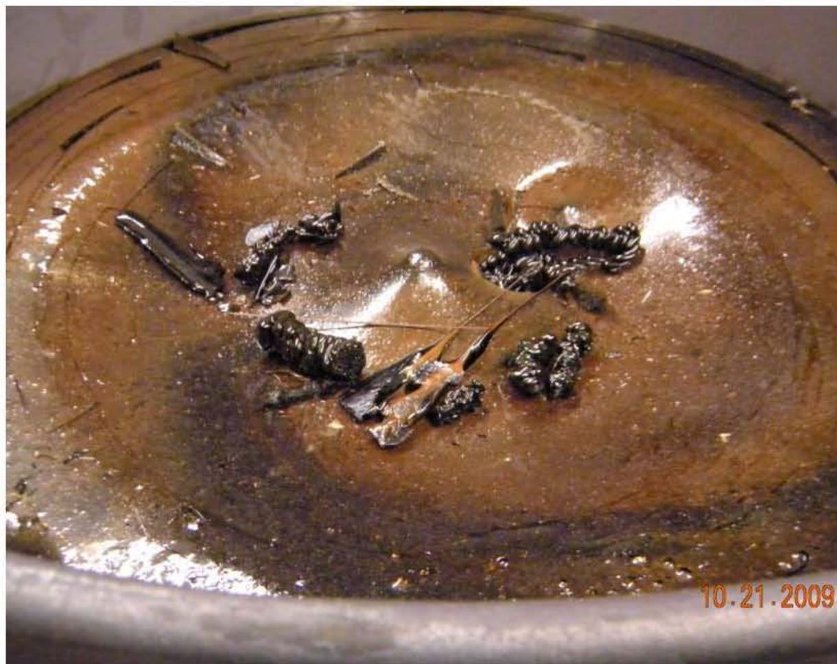
Figure 5.1. Discharge glass G-12N-151A. No foamy glass observed.
