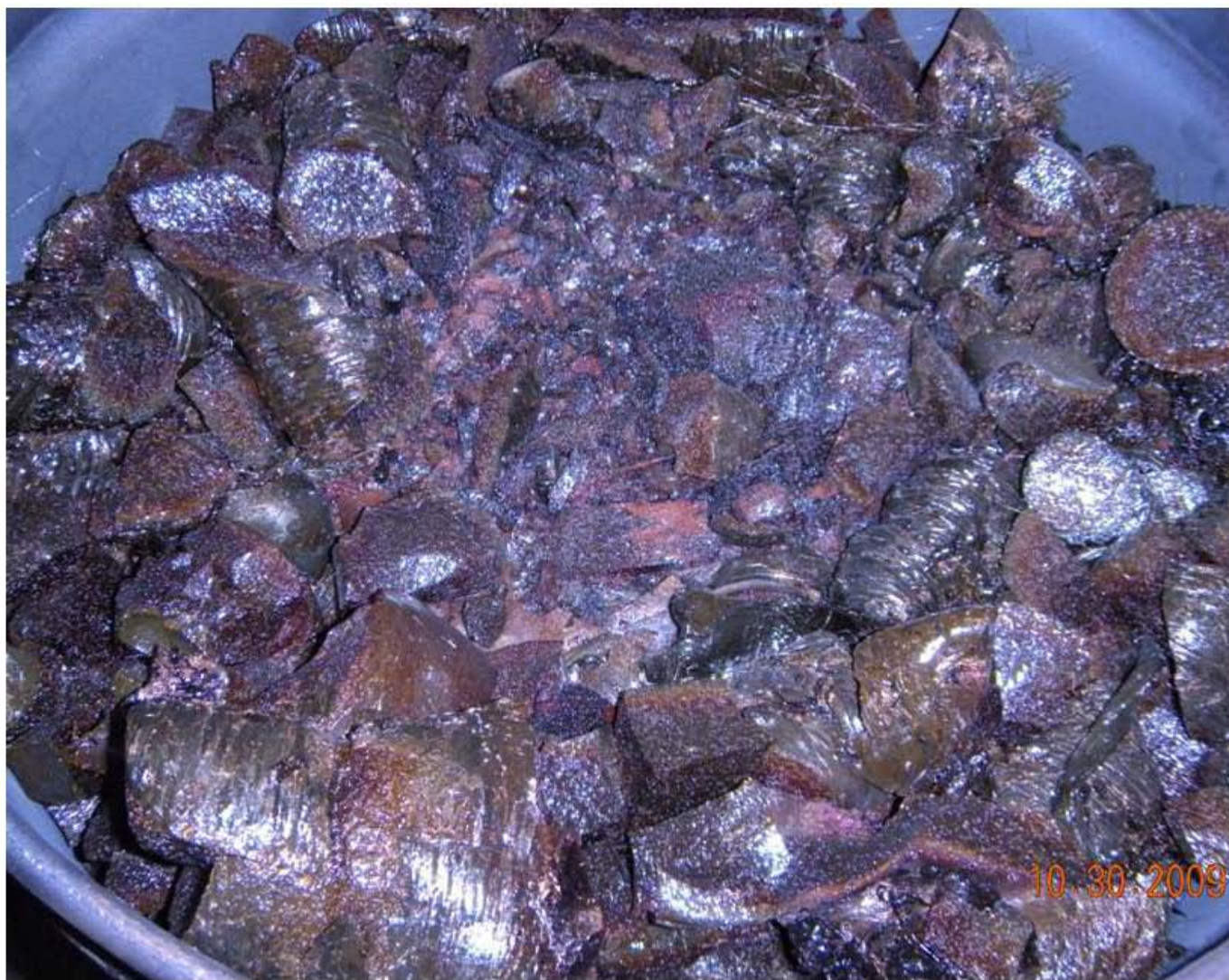
Figure 5.12. Discharge glass G-12P-72A. Foam observed.
