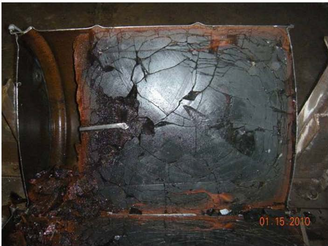
View of right half of drum, full split open, shows void around t/w.
