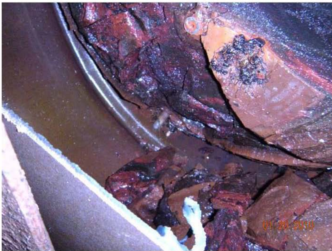
Shows cavity below surface on right half of drum, looking downward.
