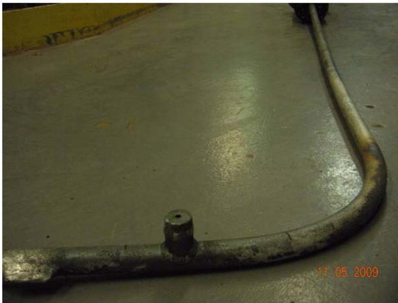
Figure 5.36. Bubbler (DB-4) after exposure to the high bismuth glass.
