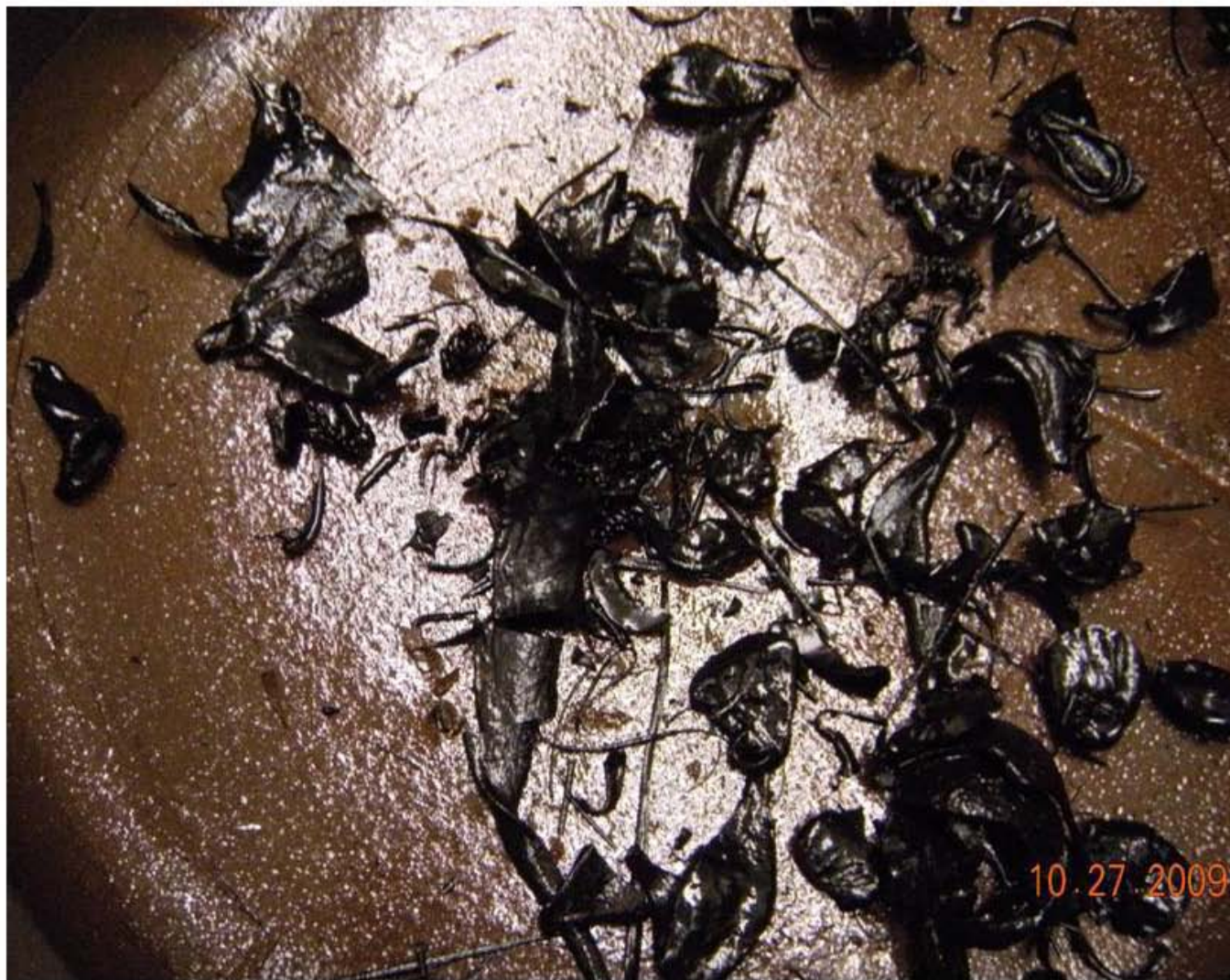
Figure 5.8. Discharge glass G12O-133A. Foam observed.
