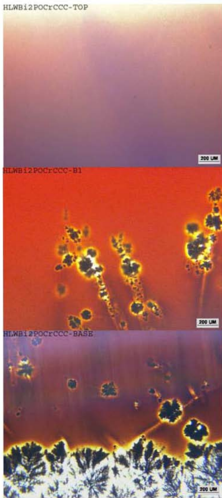
Figure 3.4s. Transmission optical microscopic images of HLW-Bi-2P0Cr after CCC.
