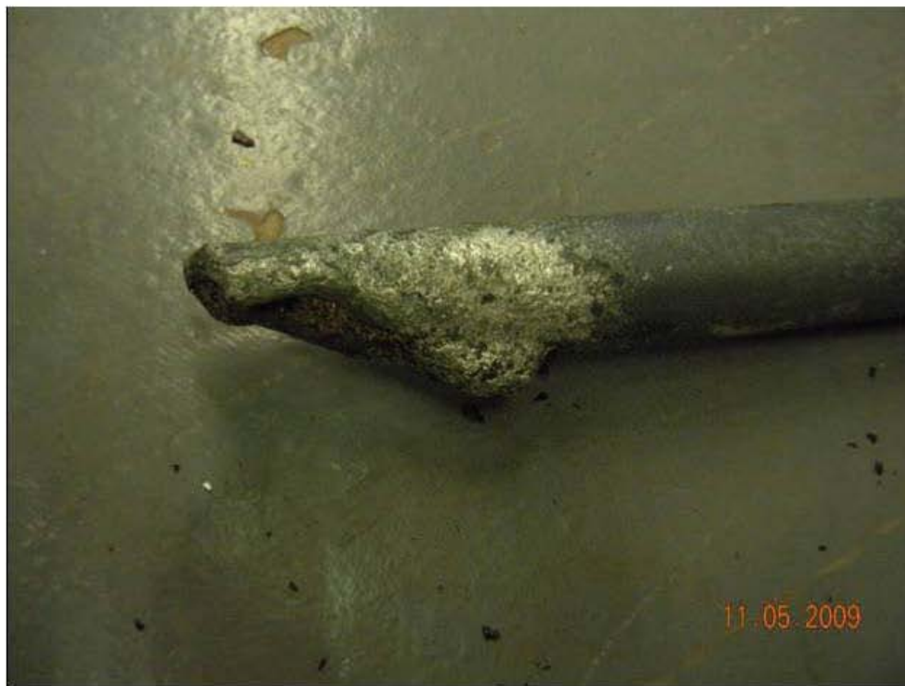
Figure 5.34. Bubbler (DB-3) tip after exposure to the high bismuth glass.
