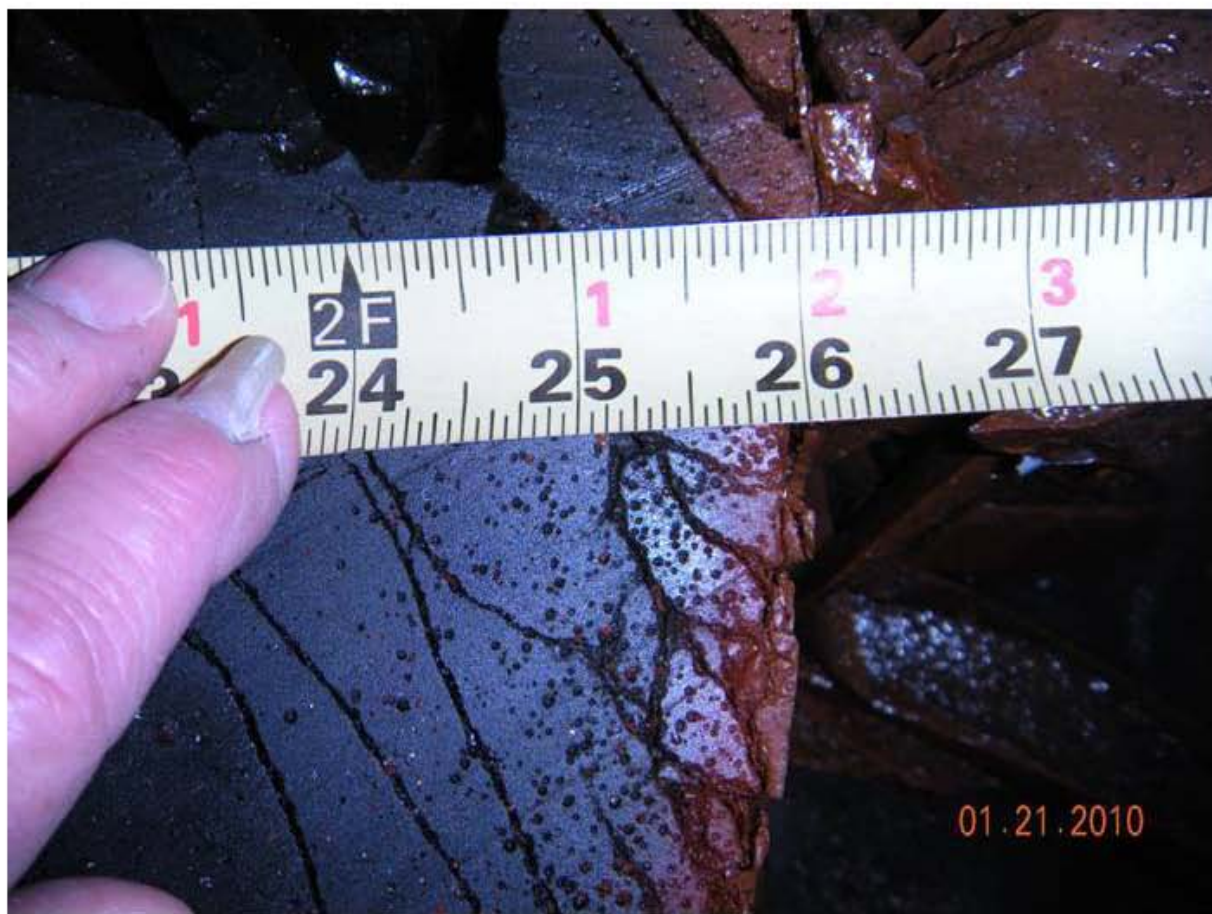
Glass measured @ 1" from left wall of right half of drum.
