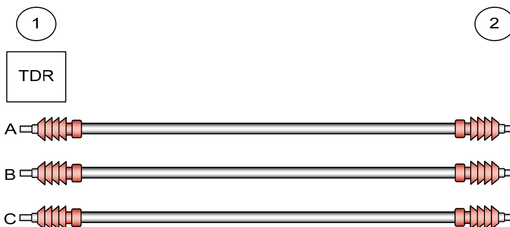
Figure 14: Three-Phase Section under Test Using TDR
