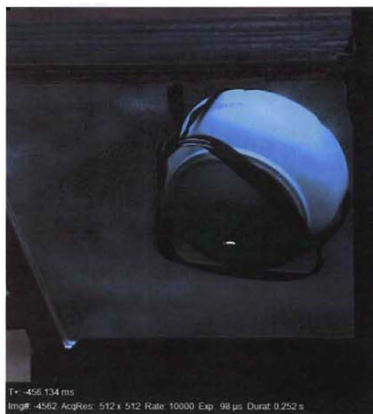
Figure 4. Hot spots and reaction spread 200 \mu s after impact onto sanded glass from 3 ft.
