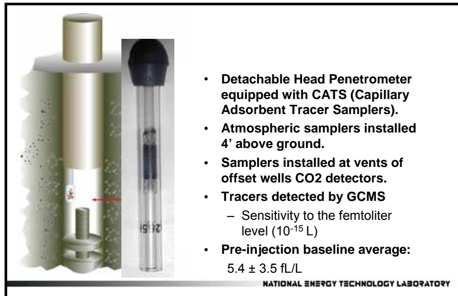
Figure 18: Tracer Soil-Gas Monitoring Penetrometers
