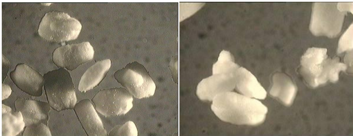
Figure 3.34 425-710 \mu\text{m} \text{Na}_2\text{CO}_3 particles before (left) and after (right) sintering at 730 °C.
