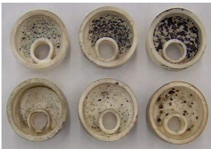
Figure 3.39 BL stains on alumina trays from BL- \text{Na}_2\text{O}\cdot 3\text{TiO}_2 mixtures after 1 hr in \text{N}_2 at 520 °C and 360 °C for top and bottom row respectively, and from left to right for 90-180, 180-425, and 425-710 \mu\text{m} particle size range respectively.
