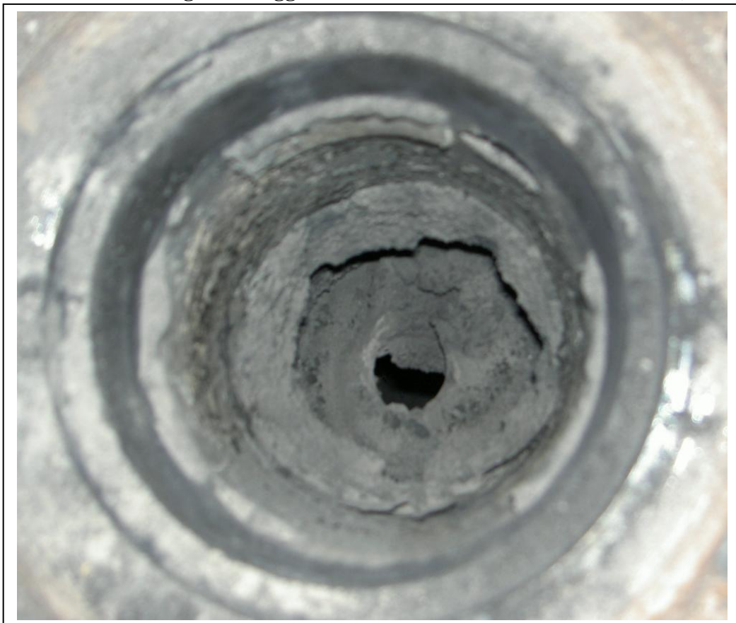
Figure 6: Agglomeration in the freeboard – one view (test #8)
