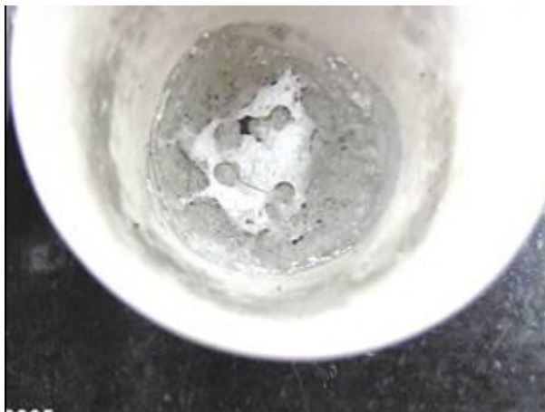
Figure 3.33: Agglomeration of BL plus \text{Na}_2\text{O} \cdot 3 \text{TiO}_2 slurry in air at 500 °C after 17 hr.
