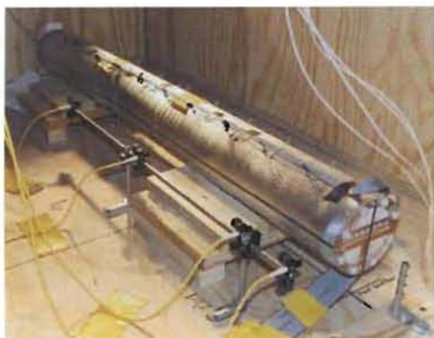
Fig. 1. Set-up of cylindrical Al confinement of ANFO (94/6 wt.% AN/FO). The ANFO/Al tube length was 914.4 mm. The ANFO ID was 76.2 mm, while the Al wall thickness was 12.7 mm.
