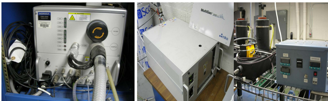
Figure 7. Horiba OBS-2200 (left) and MKS MultiGas 2030HS with FTIR (middle and right) at CAR lab used in the setup described in H.1.GN.1.
