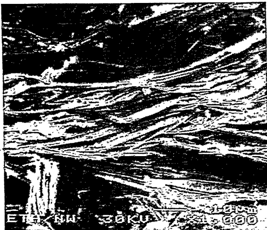
Fig.1: SEM picture of the cross-section of a Bi-2212 bulk sample processed at T_{\max}=905\text{ }^{\circ}\text{C} .
