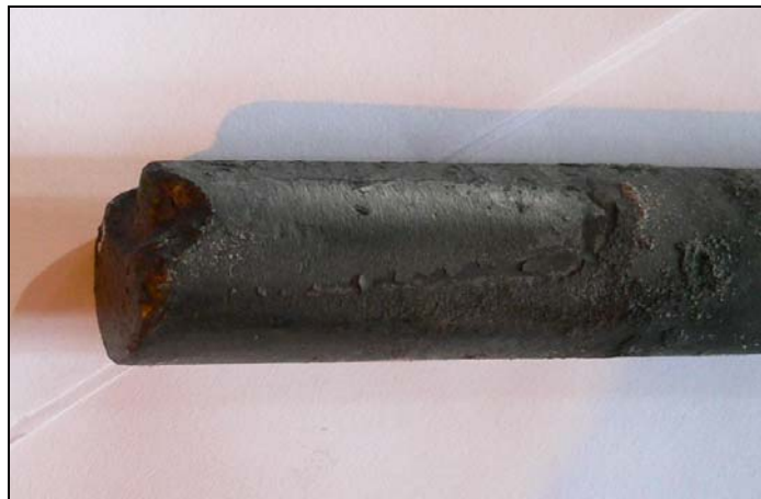
Figure 4-1. Eroded Gasifier Thermowell.
