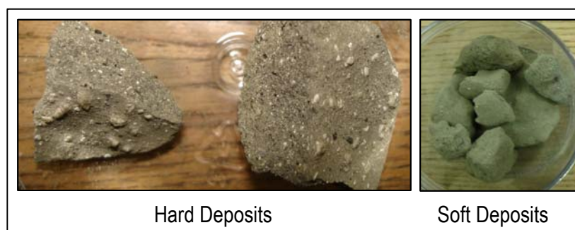
Figure 3-25. Material Removed from Lower Mixing Zone after TC21 Part B.
