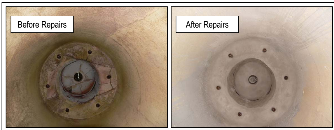
Figure 3-27. Atmospheric Syngas Combustor Before and After Refractory Repairs.
