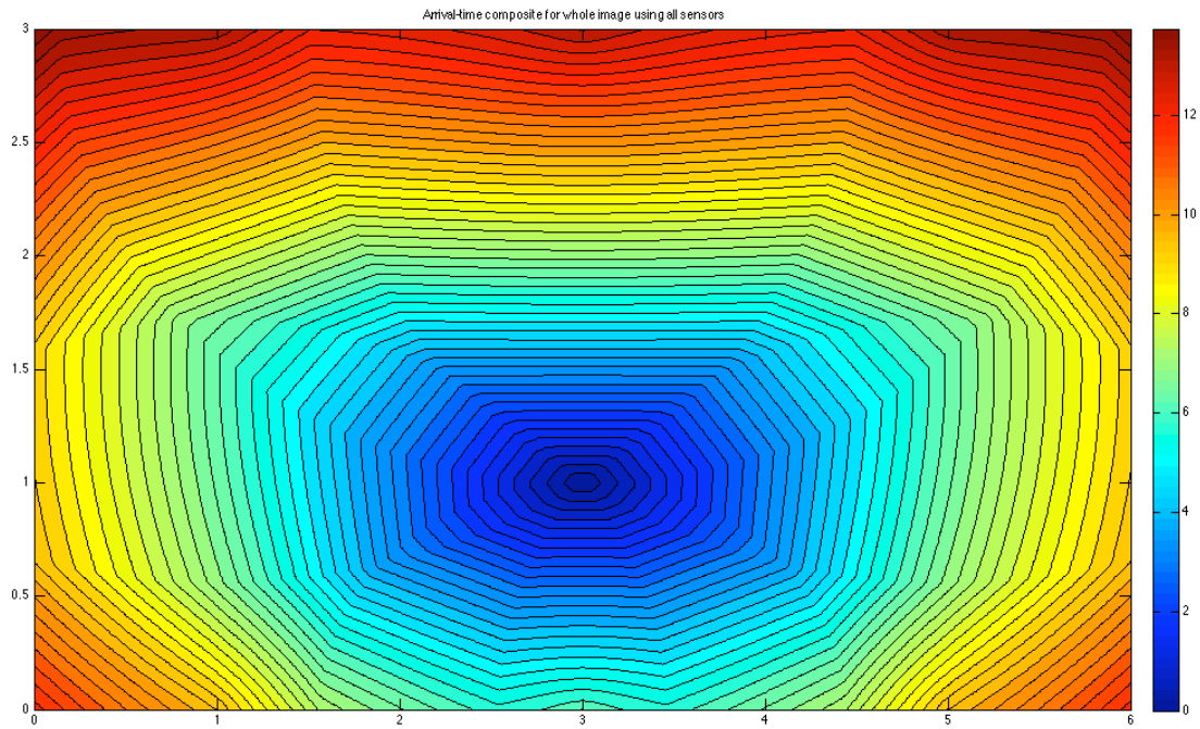
Figure B.5 - sum of the residuals for a six transducer array for a rectangular specimen with a source located at (3,1). While this is for a two dimensional case, it could easily be extended to three dimensions. This surface was calculated using a velocity anisotropy factor of 0.5.
