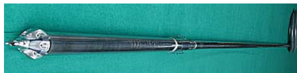
Figure 3. Instrumented Capsule for Material Irradiation Tests
