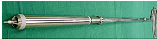
Figure 4. Instrumented Capsule for Fuel Irradiation Tests
