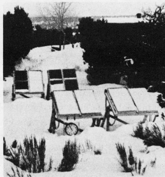
11:00: 40° PANELS PARTIALLY CLEAR, 30° PANELS STILL COVERED.
