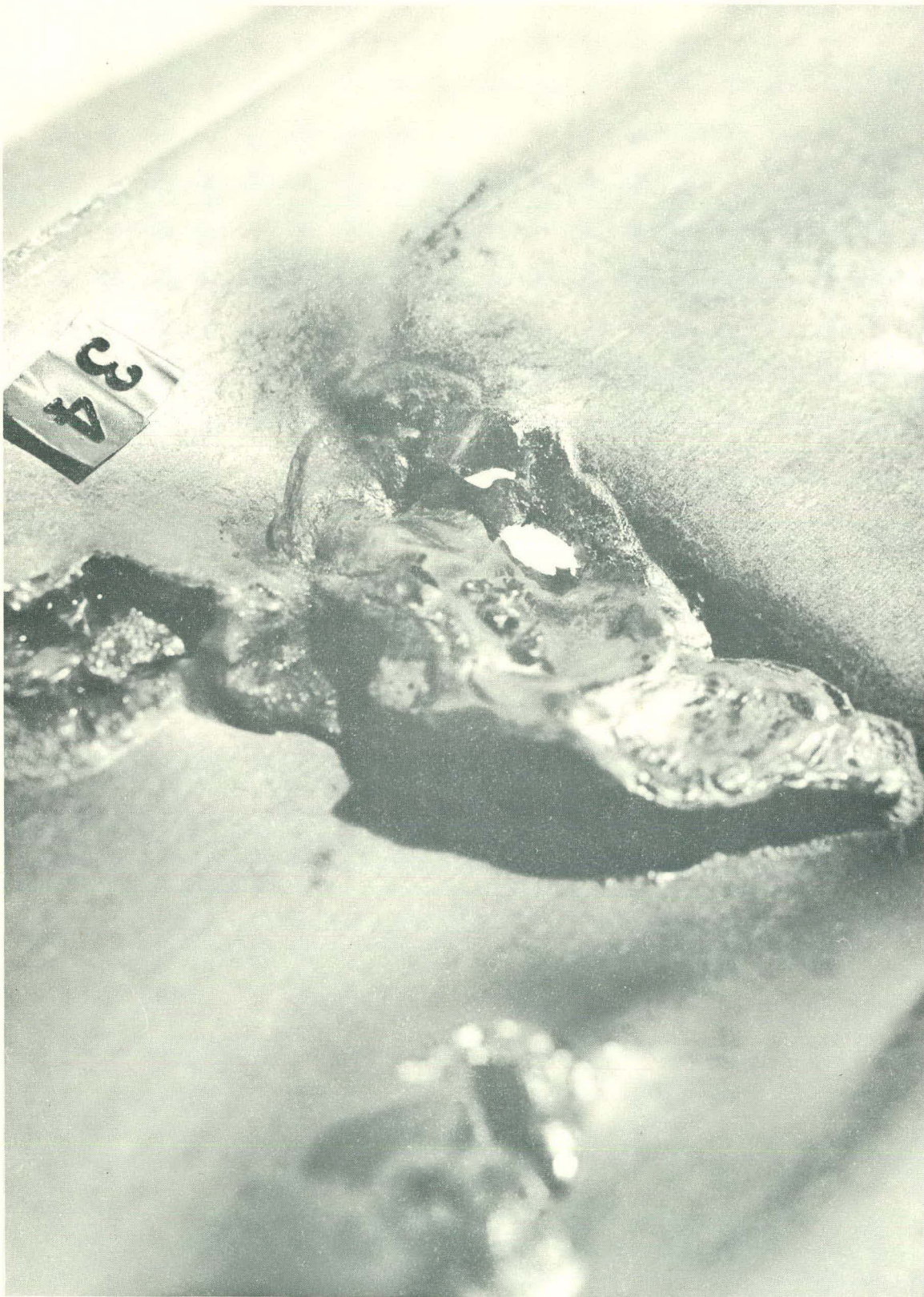
Fig. 44 Close-up view of melt showing hole through fuel plate - 5 msec test
