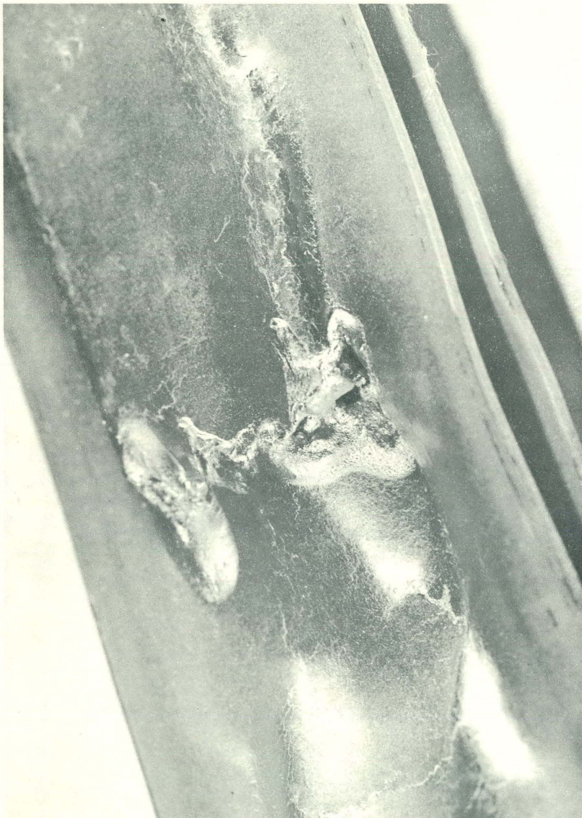
Fig. 41 Melts and fractures - 5 msec test
