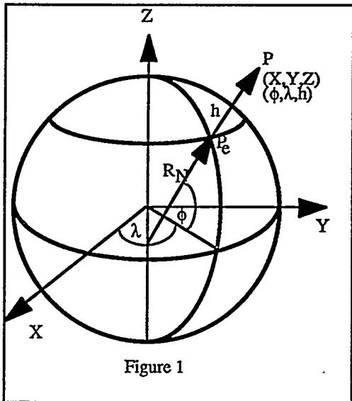
The transformation from geodetic to geocentric coordinates is straightforward<sup>18</sup> and is given by:
