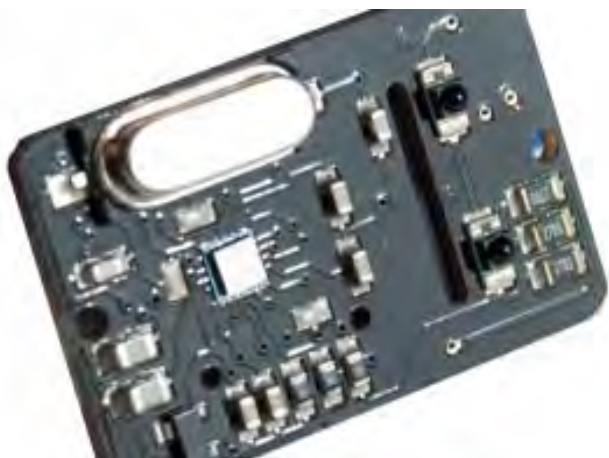
Figure 18. epc610 time of flight sensor mounted to a PCB.
