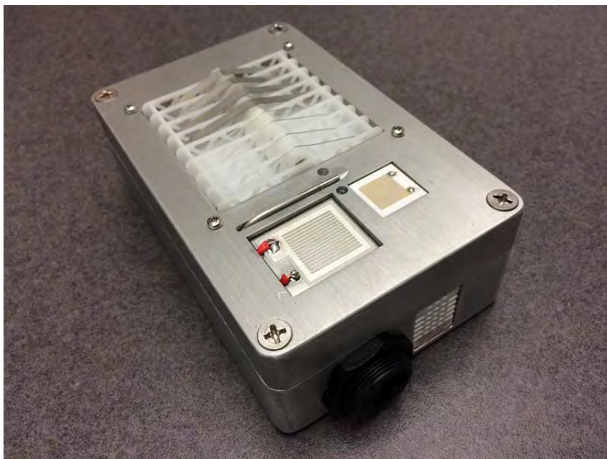
Figure 37. Assembled sensor module. A complete assembly of the sensor module included the SCC sensor, corrosion sensor, time of wetness sensor, humidity sensor, and thermocouple.
