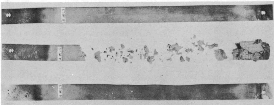
Fig. 5.14—Influence of thickness of Fe-Cr-Y alloy on oxidation resistance at 2300°F. Lightest gauge, 0.004 inch completely oxidized (Neg. U36241B)
