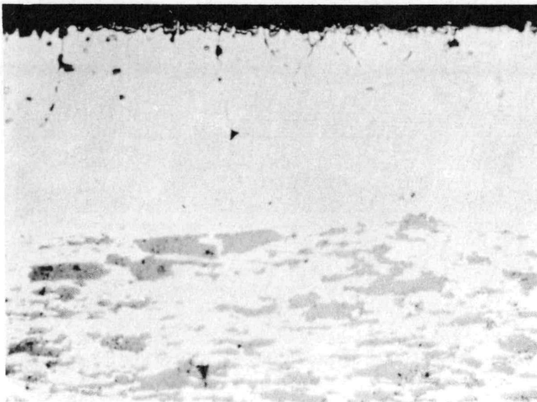
~0.002-inch intergranular attack after irradiation at 1 \times 10^3 n/cm 2 -sec for 102 hours at 1850°F
