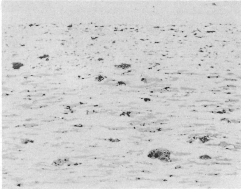
Fig. 5.10 - Cross section through typical fuel ribbon with Cr-1Ti-42UO 2 core; overlay or sub-cladding of Cr-1Y-15Y 2 O 3 adjacent core and outer cladding of clear Fe-Cr-Y alloy
