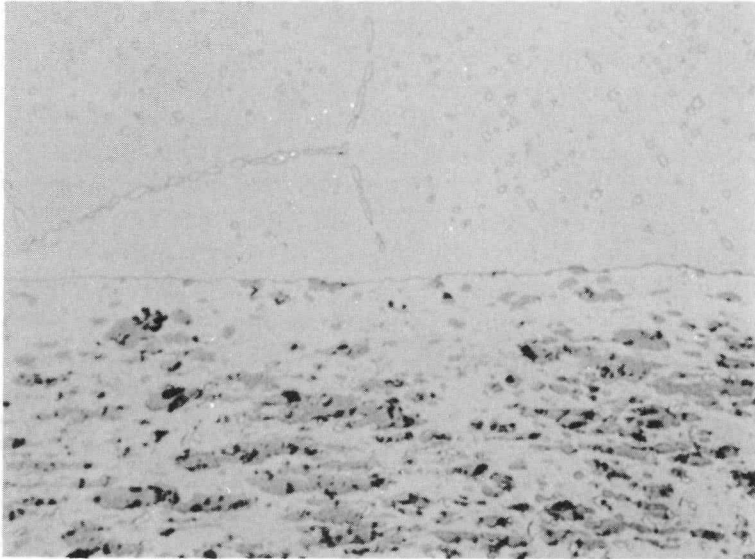
Fig. 4.3—Cross section through fuel stock—carbon deoxidized and cycled 208 hours between 2250°F and 500°F
