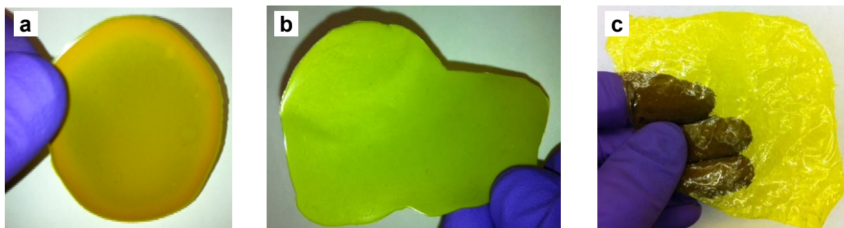
Figure 33. Photographs of PIM-1-based MMMs, (a) 11.1% (w/w) MIL-53/PIM-1 MMM, (b) 17.6% (w/w) ZIF-8/PIM-1 MMM, and (c) 11.1% (w/w) ZIF-90/PIM-1.
