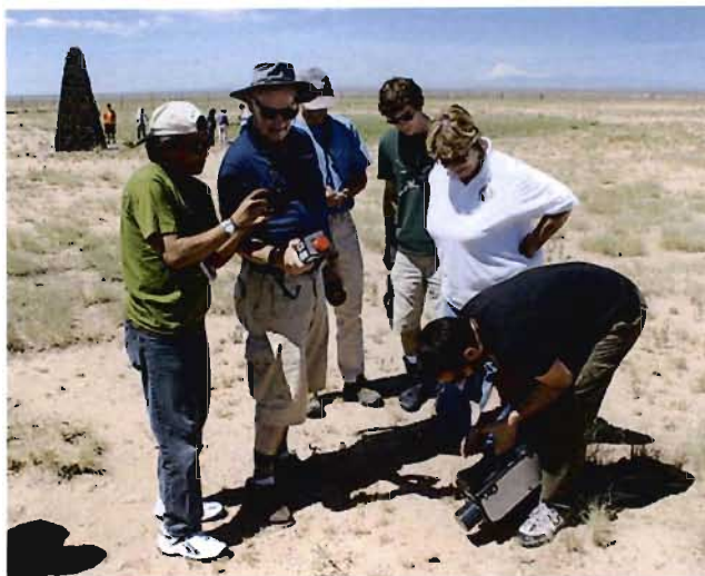
Figure 1. In Situ measurements at the Trinity Site using an identiFINDER and an Ortec microDetective. The obelisk in the background marks Ground Zero, where remnants of the steel tower are still visible today.
