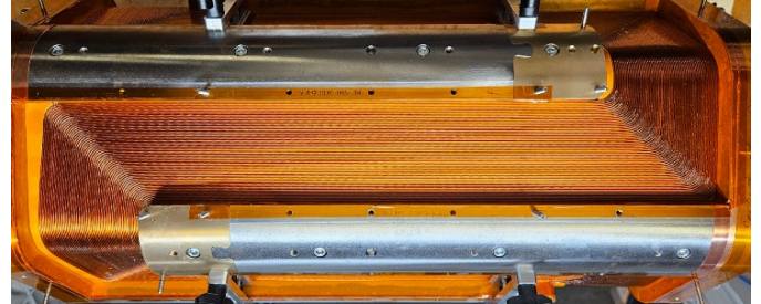
Fig. 10. The 8th layer of the full-size MARS-D CLC
