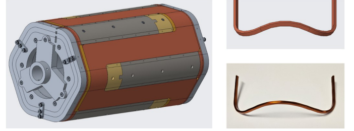
Fig. 4. Winding setup and conductor bending
