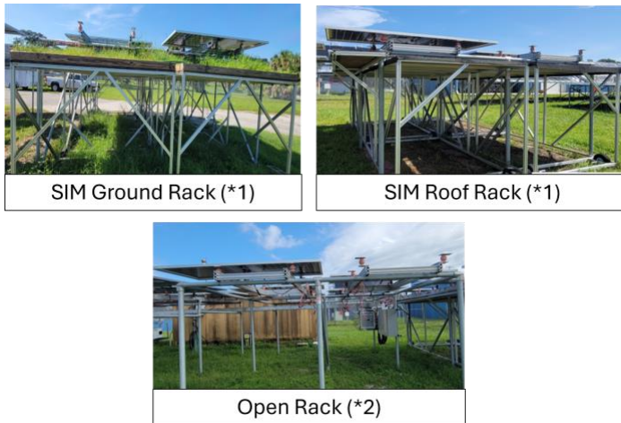
Fig. 1: Pictures of the three mounting configurations on the HV testbed (4 racks in total).
