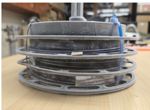
Figure 18. Bare optical fibers looped around custom 3D-printed wheels after completion of cryogenic cycling. Each wheel has a diameter of 16 cm and a height of 2 cm, allowing the fiber to complete two loops with a controlled bend radius. The wheels were mounted on the movable arm of the CTCA and repeatedly immersed in liquid nitrogen as part of the thermal cycling procedure.
