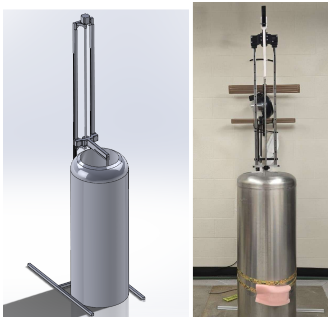
Figure 17. Cryogenic Thermal Cycle Apparatus (CTCA) used to test the optical fibers components under thermal stress. The setup includes the structural aluminum frame, 3D-printed support components, and the cryostat filled with liquid nitrogen, which allows for repeated thermal cycling of optical fiber assemblies.
