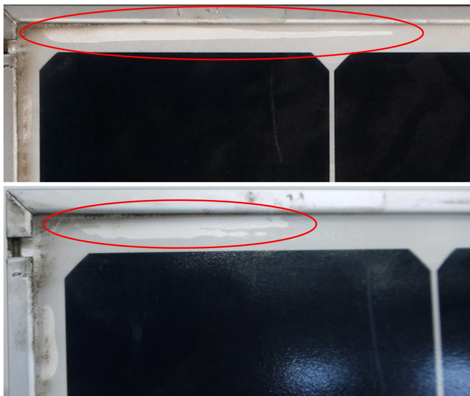
FIGURE 14 | Detailed photographs of a PV module with delamination between encapsulant and backsheet at the module edge; after field-ageing (top) and subsequent accelerated aging (humidity-freeze, bottom).
