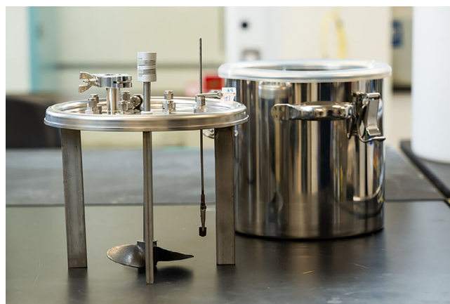
FIGURE 1 A photograph of the 8-port stirred-reactor coupon analysis (SRCA) reactor used in the interlaboratory study (ILS). The image shows the lid, propeller, baffles, and a glass coupon in the foreground. This combination of pieces is placed in the stainless-steel reactor shown in the background. The inner dimension of the reactor is 23.8 cm diameter and 23.8 cm in height.
