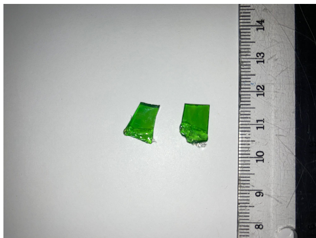
FIGURE 2 Examples of masked coupons before stirred-reactor coupon analysis (SRCA) testing. The ruler scale is in centimeters with millimeter demarcations.
