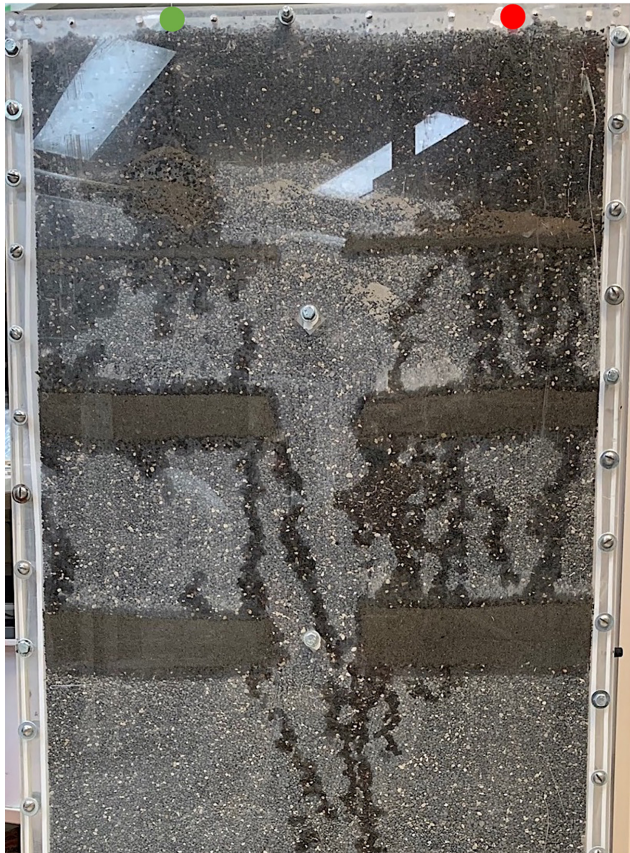
Figure 5. Qualitative comparison of groundwater infiltration (left side) showing predominantly flow around the low permeability inclusion or an anionic surfactant (right side) showing flow through and around the low permeability inclusion. Groundwater infiltration at top left green dot and surfactant infiltration at top right red dot.
