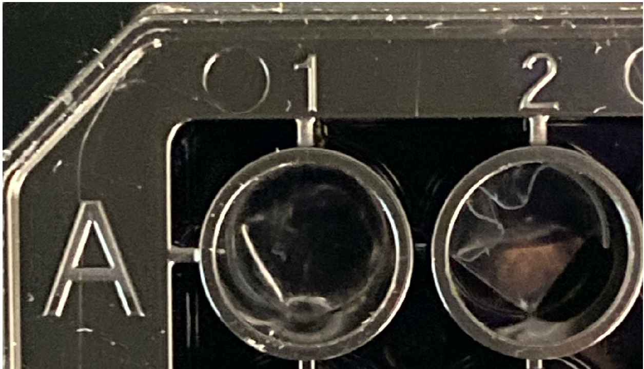
Supplementary Figure 2: Overview of correct and incorrect film orientation for NBD-H LDPE assays. The film on the left, in well A1 was correctly cut, using the bore end of a 200 \mu L pipette tip. The film on the right, in well A2 was cut as a 5 mm x 5 mm square that leads to high error in the NBD-H assay.
