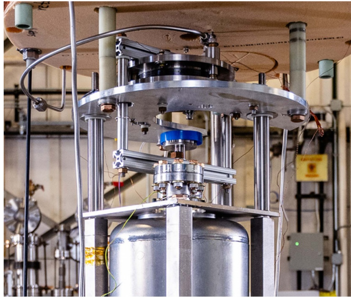
Figure 7. Fine tuning of cavity using a pneumatic bellows tied to the QWR center conductor.
