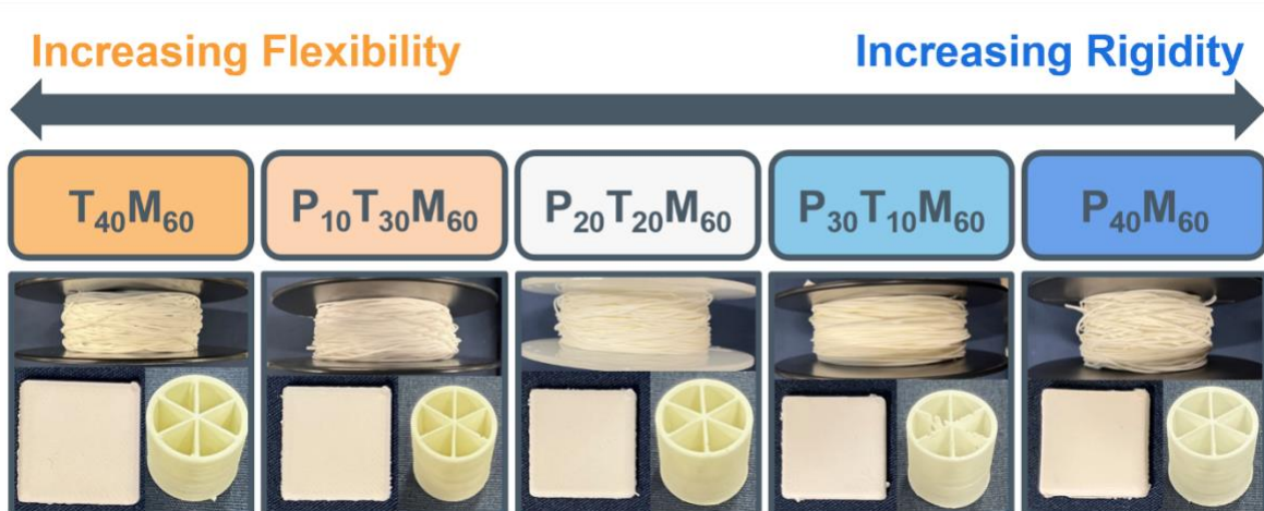
Figure 1. MEPCM composite materials ranging from more flexible (TPU) to more rigid (PCL) at a constant MEPCM ratio of 60 wt.% and 40 wt.% polymer. Each subscript denotes the weight percentage with T – TPU, P – PCL, M – 6D MEPCM. Below each ratio are images of the extruded filament, 100% rectilinear infill test squares (20 mm x 20 mm x 2 mm rectangular prism), and 10% triangle infill cylinder (15 mm diameter, 15 mm tall cylinder) to assess initial print conditions and behaviors of composite materials.
