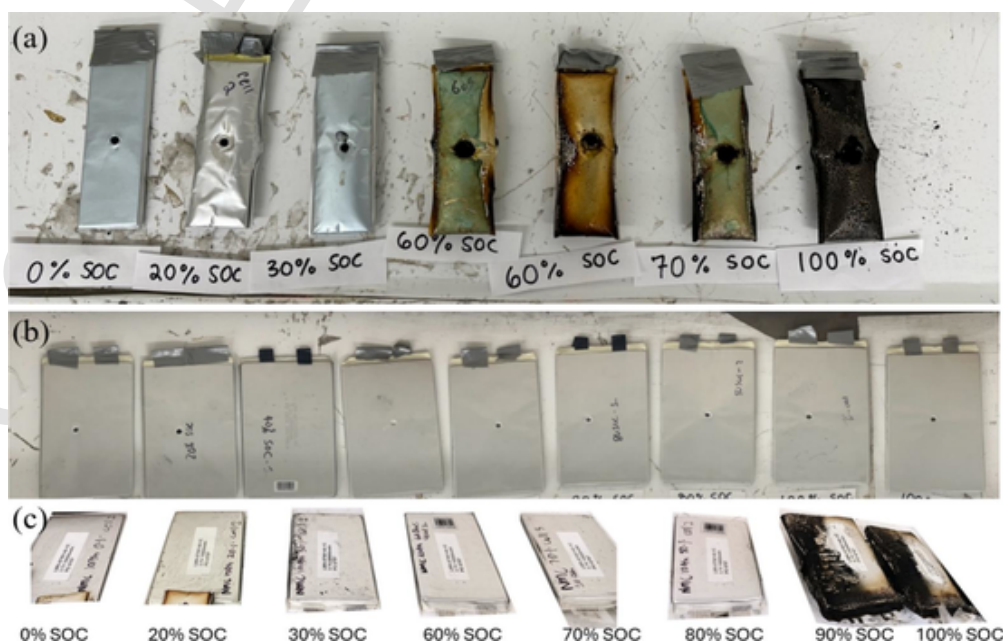
Fig. 9. Cells after indentation test, (a) LCO 4 Ah cells, (b) LFP 15 Ah cells, (c) NMC 10 Ah cells.
