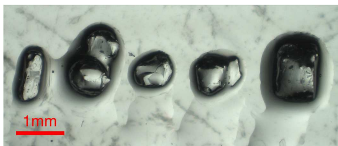
Figure 1: Crystals of \text{Rb}_3\text{Tb}(\text{PO}_4)_2 suspended in immersion oil; dark portions of the crystals are due to shadows resulting from the oil, the size of the crystals, and the angle of the light
