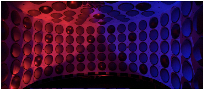
FIG. 3. Interior view of the CCM200 detector during assembly. The fiducial region, enclosed by the PMTs and support structure, encompasses 7 tons of LAr. The PMTs protrude 6.2 mm into the fiducial volume, providing full photocathode exposure. The reflective PMTs do not have wavelength shifter coating while the matte PMTs are coated in TPB. 20% of the PMTs are uncoated for a total of 40 uncoated PMTs.
