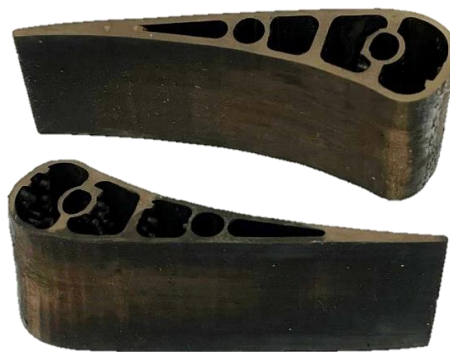
Fig. 2 Additively manufactured ceramic turbine vane.
