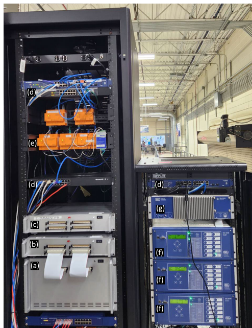
FIGURE 8. The implemented HIL testbed, which consists of (a) Typhoon Power Amplifier, (b,c) two Typhoon HIL 604 working in parallel, (d) Netgear network switches, (e) DER protocol translators, (f) SEL 651 R, and (g) SEL 3355 industrial computer.
