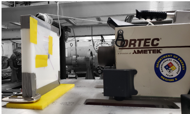
FIG. 8. The picture of \gamma -ray peak measurement with portable HPGe detector. The distance from ^{235}\text{U} target to the detector was 22 cm.
