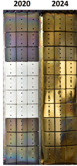
Figure 6. Example of IB surfaces with BN tiles after installation in 2020 and before removal in 2024.
