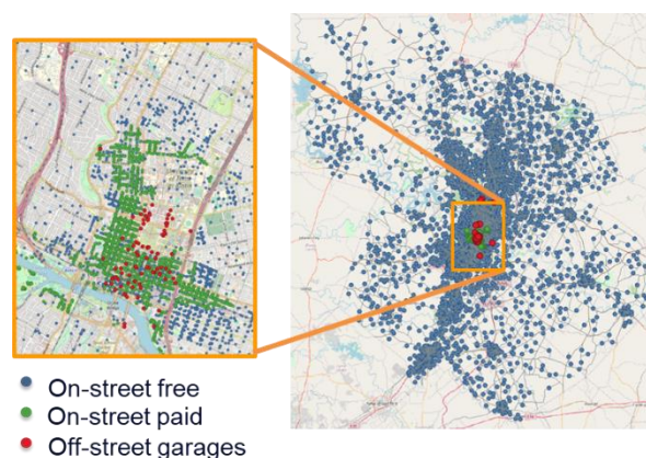
Fig. 1. On-street and Off-street Parking Locations and Lots for SAV Use, as Simulated across the 6-County Austin, Texas Region
